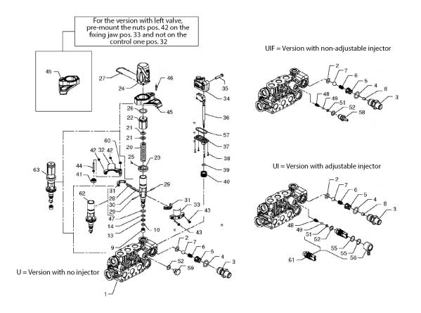
\* When assembling apply petroleum based grease
