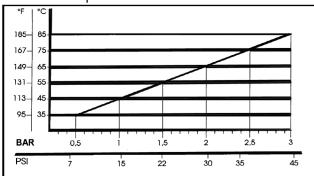
Naturally, if the application allows for feeding the pump with 45 psi (3 bar) even at low temperatures (for example: 115° F/45° C the life of the wet end of the pump will be even longer.
