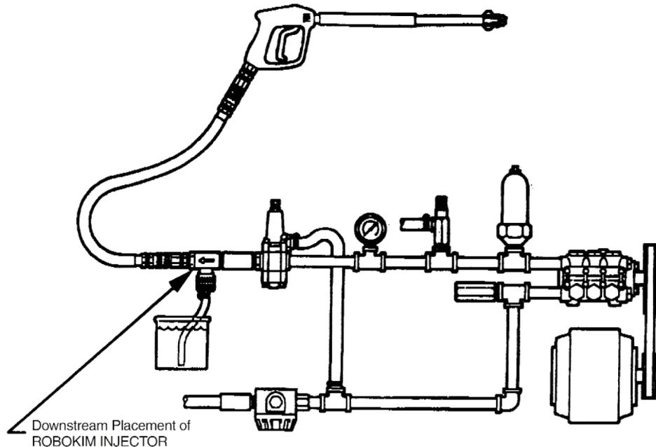
Be sure that this accessory as well as all other components exceeds the system's maximum pressure rating. The system's output flow must be within the volume specification of this chemical injector for proper system operation and acceptable back pressure.
