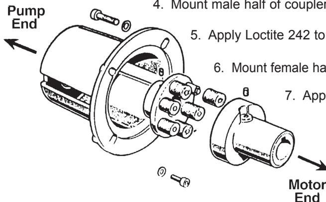
5. Apply Loctite 242 to threads of set screw and tighten.
