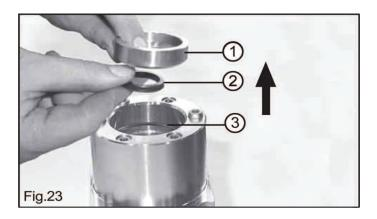
Remove the rear seal support 1, the rear seal, 2 and the o-ring, 3. Fig. 23.
