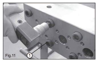
Loosen and remove the 8 head screws (1, Fig. 11).
