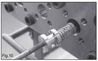
Once removed take out the delivery valve guide with the spring and valve poppet. AN M10 threaded bolt to be used as a simple extractor would help the operation (see Fig. 10).
