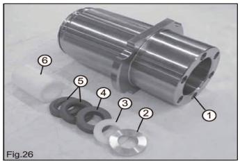
Reassemble packing support and cylinder, Screws 1, Fig 26 should be tightened with a torque wrench set for 4 lbs. Fit each new component of the pressure packing set in the cylinder making sure of the correct order as shown in Fig. 26 and Fig. 27:
