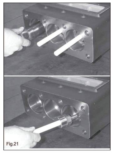
Once the cylinders are removed, loosen the plungers and check them for wear (Fig. 21). Replace if necessary.
