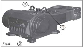
If necessary, top up from the oil plug (3, Fig. 8).
