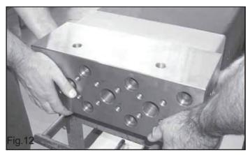
Remove the pump head (1, Fig. 12).
