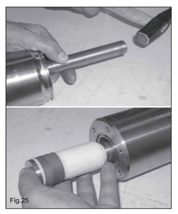
Insert a pin of adequate dimensions and smartly tap until the complete pressure packing set is out (Fig. 25). Replace pressure packing set at every inspection.
