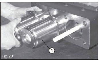
Once head and collector are removed the cylinders are free to be taken out of the crankcase. Tapping the cylinders all around with a plastic hammer helps to loosen them from possible scaling or deposit accumulated during operation. When removing the cylinders take their weight into account and pay attention not to hit and damage the plungers.
