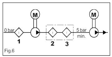
The filters should be installed as close as possible to the pump, allow easy inspection and have the following specifications:
