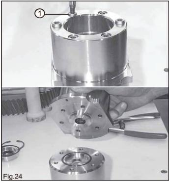
Remove the 6 packing support screws (1, Fig. 24).
