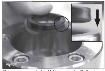
The new rear seal should be mounted with the larger diameter side first in, as shown in Fig. 29.
