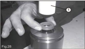
Each pressure packing set component should fit tight in the cylinders. A pin of adequate dimension (1, Fig. 28) helps in guiding each component straight and aligned all the way down the cylinder.
