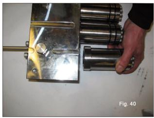
• Take out the M8 x 100 screws fastening the liners to the head as shown in fig. 39 and proceed as shown in fig. 40.
