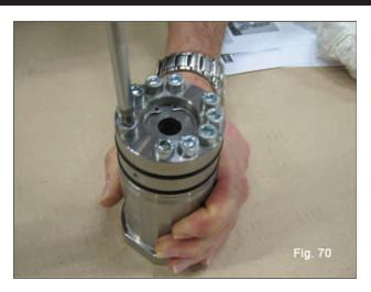
Assemble the LP and HP seals support units - liner manually screwing the screws M6 x 80 as indicated in fig. 70. Then proceed with calibration using a torque wrench as indicated in Chapter 3.
