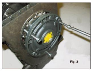
push the plunger guides forward with their con-rods to facilitate side extraction of the pump shaft. There are two reference points visible on the shaft (indicated with 1 in fig. 4 and in fig. 4a). These must be turned toward the operator to facilitate extraction.
