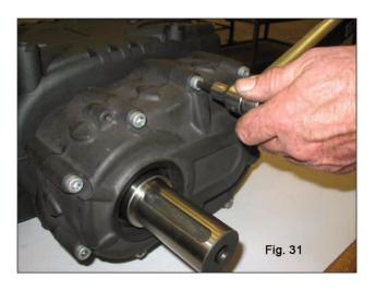
Check the conditions of the pinion oil seal lip; if it needs replacing, position a new pinion oil seal ring using the tool p/n F27904800.
