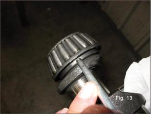
The new bearings can be mounted cold with a press or rocker, supporting it on the lateral surface of the ring nuts involved in press fitting with the rings. The press fitting operation can be facilitated by heating the involved parts to a temperature between 250°F-300°F (120°C-150°C), ensuring that the ring nuts fit into their seats.
