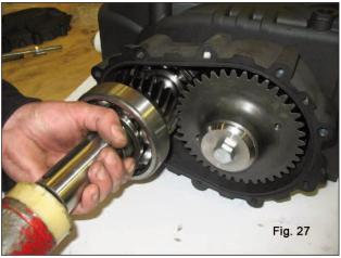
The bearings and crown wheel can be mounted cold. The press fitting operation can be facilitated by heating the involved parts to a temperature between 250°F and 300°F (120°C and 150°C), ensuring that the ring nuts fit fully into their seats.
