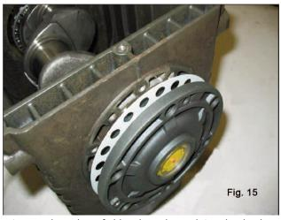
Once the type and number of shims have been determined using the table, check the following: assemble the shim pack on the indicator side cover centering (fig. 15), secure the cover to the casing, following the procedure in 2.1.2 and tighten the screws to their recommended torque.
