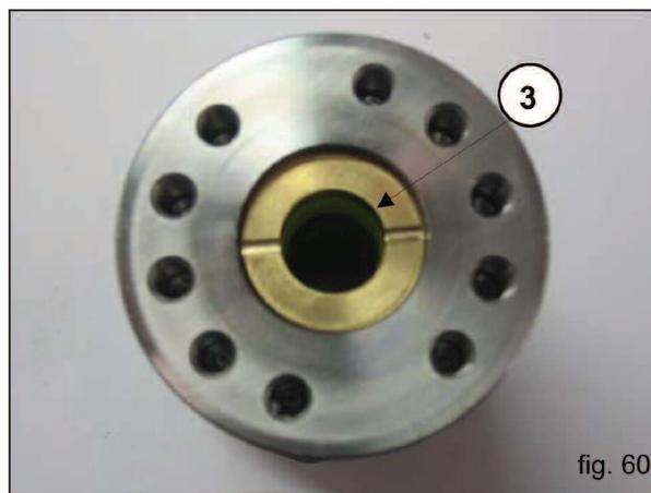
C) Insert the anti-extrusion ring (2) and the seal bushing (3) positioned as per figs. 59, 60 and 61.
