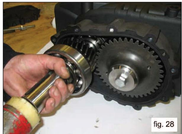
The bearings and the ring gear can be mounted cold. The press fitting operation can be facilitated by heating the involved parts to a temperature between 250° - 300° F (120° - 150° F), ensuring that the ring nuts go down to end stroke in their housings.
