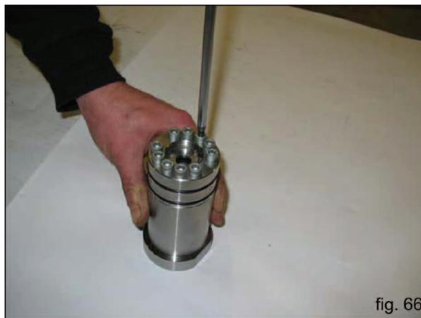
E) Assemble the support unit - liner, manually screwing in the M6x40 screws as indicated in fig. 66, then proceed with calibration with a torque wrench as indicated in Chapter 3.
