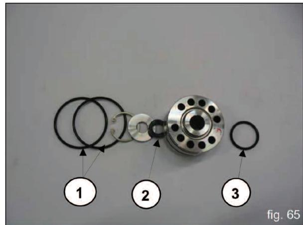
D) Replace the seal support unit as indicated in fig. 64 and 65 replacing components 1,2 and 3.
