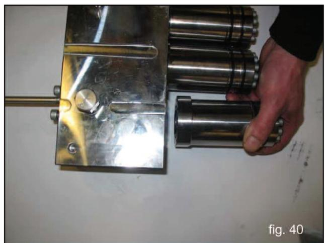
D) Remove the M8x100 head liner fixing screws as indicated in fig. 39 and proceed as indicated in fig. 40.
