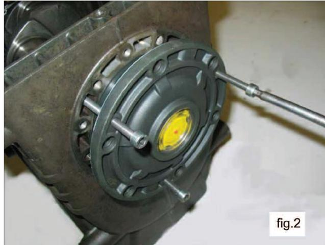
Push the plunger guides forward with their con-rods to facilitate side extraction of the pump. there are two reference points visible on the shaft, 1, as shown in fig. 3 and in fig. 3a. These must be turned toward the operator to facilitate extraction.
