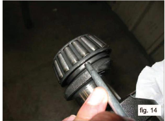
The new bearings can be mounted cold with a press or rocker, supporting it on the lateral surface of the ring nuts involved in press fitting with the rings. The press fitting operation can be facilitated by heating the involved parts to a temperature between 250°-300° (F) 120°-300° (C), ensuring that the ring nuts go down to end stroke in their housings.
