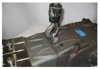
In case of disassembly, to avoid letting dirt inside the front part of the crankcase, close the threaded hole with the appropriate cap, supplied.
