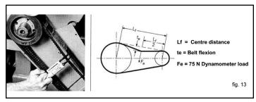
Note: If not differently indicated by the belt manufacturer, the inspection of the correct tension value, and the related tension adjustment if needed, is to be carried out after at least 30 minutes of operation in order to obtain belt settling. The best efficiency and maximum duration is obtained with a correct tension value.
