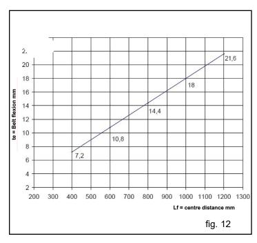
Conclusion: using a dynamometer, by loading the belt with 75 N as indicated in fig. 13, you will obtain a flexion value "te" of about 10.8 mm.
