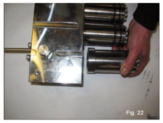
• Take out the M8 x 100 screws fastening the liners to the head as shown in fig. 21 and proceed as shown in fig. 22.
