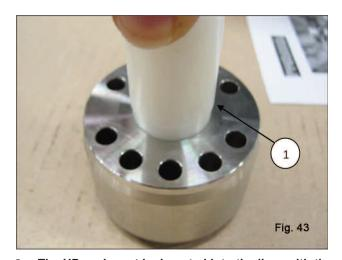
The HP seal must be inserted into the liner with the energizing O-ring in the working direction of the plunger as shown in fig. 42 and fig. 44. Before inserting them into their seats, the HP seals must be lubricated with silicone grease Type OKS 1110, following the operations listed below: A) The external diameter must only be slightly greased;
