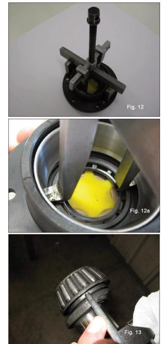
The new bearings can be mounted cold with a press or rocker, supporting it on the lateral surface of the ring nuts involved in press fitting with the rings. The press fitting operation can be facilitated by heating the involved parts to a temperature between 250°F-300°F (120°C-150°C), ensuring that the ring nuts fit into their seats.
