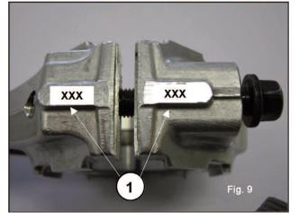
Fasten the caps to their respective con-rod shanks by means of M8 x 1 x 48 screws (fig. 10) lubricating both the underhead and the threaded shank, proceeding in two different stages:
