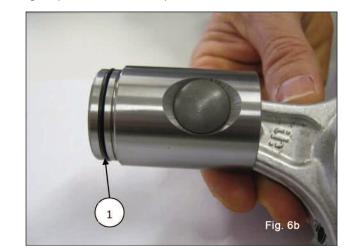
Insert the plunger/con-rod guide units into the pump casing, directing the numbering on the con-rod shank towards the top of the casing.
