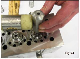
If the valve seats are blocked on the head due to the formation of scale or oxide, they must be freed by inserting the tool (p/n F27508000) into the inlet hole and operating as in fig. 42.
