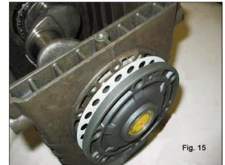
Once the type and number of shims have been determined using the table, check the following: assemble the shim pack on the indicator side cover centering (fig. 15), secure the cover to the casing, following the procedure in 2.1.2 and tighten the screws to their recommended torque.
