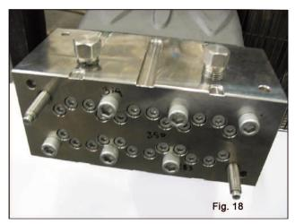
Unscrew the M12 x 260 head fixing screws No. 5 and No. 6 as shown in fig. 17 replacing them with two service pinscrews (p/n F27508200) as shown in fig. 18, then remove the remaining screws.
