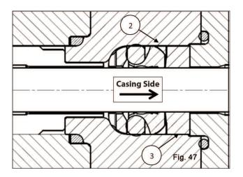
Insert the anti-extrusion ring (2)2 and the gasket bushing (3) arranged as shown in fig, 45, 46 and 47.
