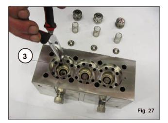
• Extract the outlet plates, 3, and their guides, 4, with the springs, as shown in fig 26 and fig. 27, check for wear and replace if necessary, and in any case within the times indicated in the "Preventive Maintenance" table of Chapter 11 in the Owner's Manual.
