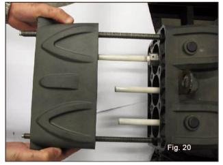
• Separate the head and the spacer for the liners from the pump casing as shown in fig. 19 and fig. 20.
