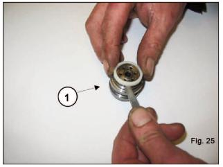
• Extract the valve seats, 1, as shown in fig. 25, check the various components for wear and replace them if needed.
