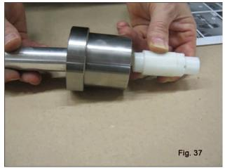
At each disassembly, the high pressure packing, 4, \ fig 35, must be replaced.
