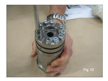
Assemble the LP and HP seals support units - liner manually screwing the screws M6 x 80 as indicated in fig. 52. Then proceed with calibration using a torque wrench as indicated in Chapter 3.
