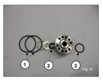
• Reassemble the seals support unit as shown in fig. 50 and fig. 51, replacing components 1, 2, and 3.
