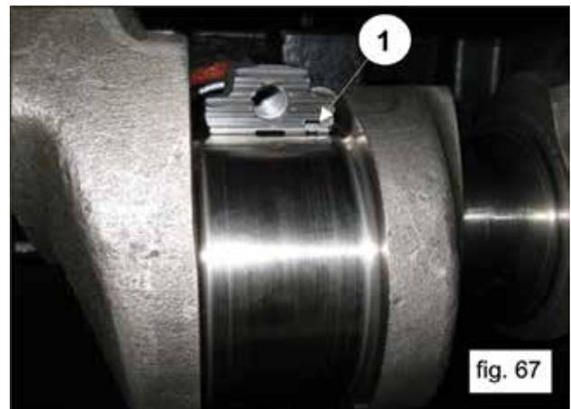
Apply the lower half-bearings to the caps (1, fig. 68) ensuring that the half-bearing reference notches are positioned in their housing on the cap (1, fig. 68).
