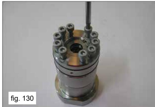
Assemble the L.P. and H.P. seals support units. – liner manually screwing the screws M8x100 as indicated in Fig. 131. Then proceed with calibration using a torque wrench as indicated in Section 3 "Screw Tightening Calibration".
