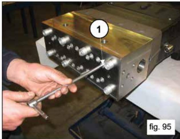
Unscrew two diametrically-opposite M16 x 80 head fixing screws (1 and 2, fig. 96) and replace them with two service pin-screws (part #F27540200)(1, fig. 97), and then proceed to remove the remaining screws.
