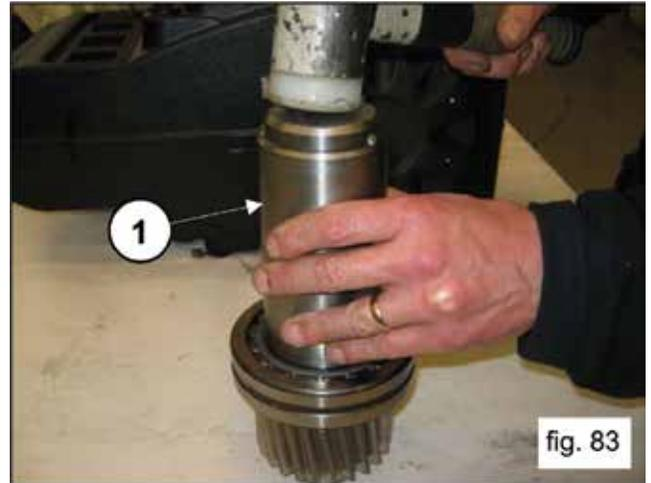
Insert the bearing support ring (1, fig. 84) and position the Seeger ring  $\varnothing 55$  (1, fig. 85).
