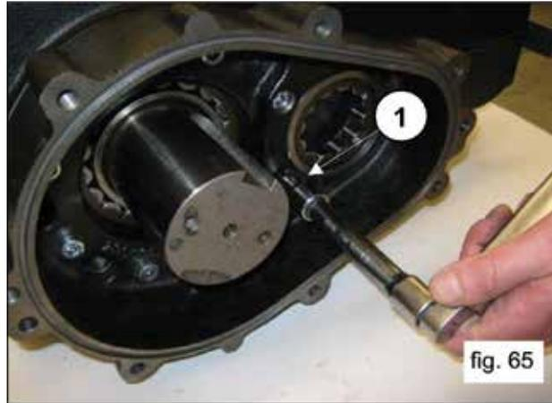
Remove the tool for blocking the connecting rods tool part #F27566200 (1, fig. 32)
