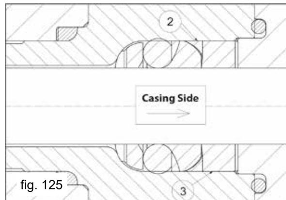
Insert the anti-extrusion ring (2, fig. 123) and the gasket bush (3, fig. 124) arranged as shown in fig. 125.
