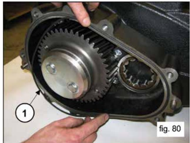
Complete assembly of the pinion on the reduction gear cover, proceeding as follows:
