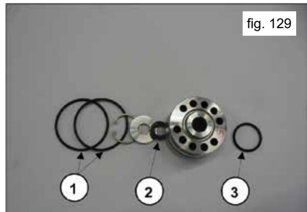
Reassemble the seals support unit as shown in Fig. 128 and 129 replacing components pos. 1, 2, 3.
