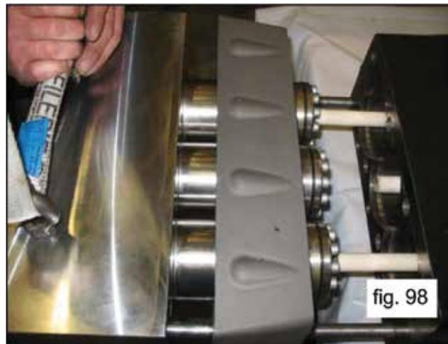
Remove the spacer for pump casing liner from the liner units (1, fig. 99).
