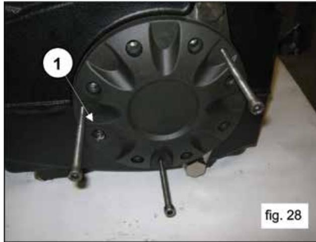
Slowly screw in the 3 M8 screws (1, fig. 29) to prevent the cover from tilting too far and getting locked in the housing. Remove the bearing cover while supporting the shaft to prevent damage. (1, fig. 30).
