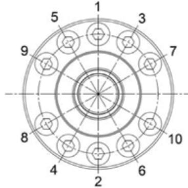
**M80x50 screw tightening according to the following sequence:
