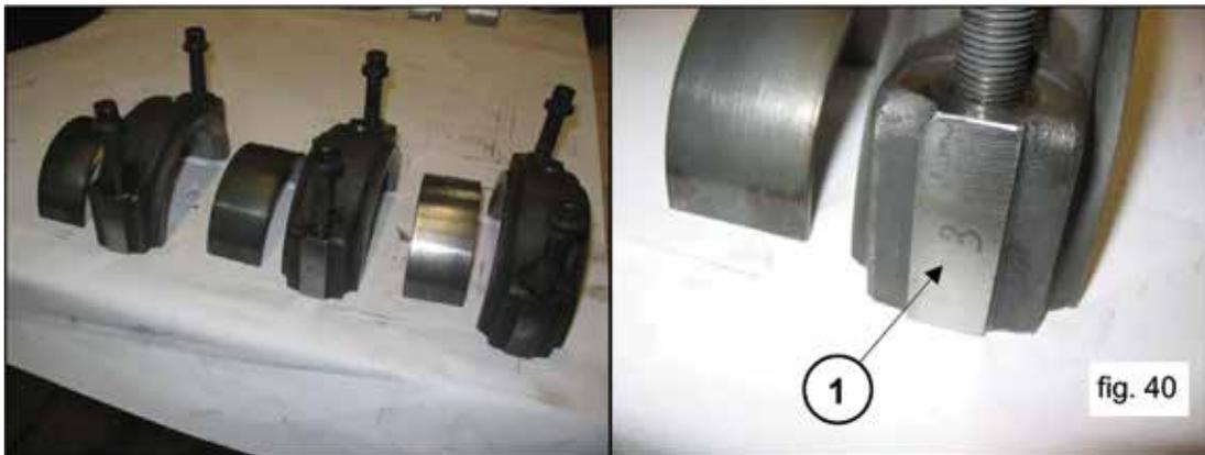
To separate the rod from the plunger guide, unscrew the hexagonal head M6 screws with a wrench (1, fig. 41).
