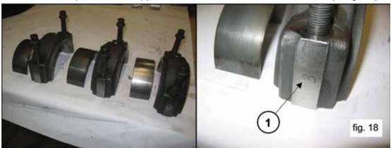
Advance the half supports completely in the direction of the hydraulic part to allow the crankshaft to come out. To facilitate this operation, use special too part #F27566200 (1, fig. 19).
