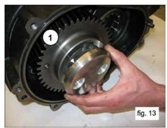
Remove the ring gear (1, fig. 14). Where necessary, it is possible to utilize an extractor hammer to be applied on the (2) M8 holes (2, fig. 14).
