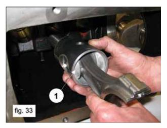
It is now possible to disassemble the plunger guide seal rings, taking care to not damage the plunger guide sliding rod.
