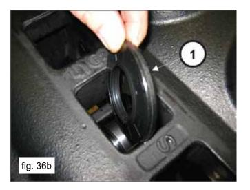
Remove the two spindle locking Seeger rings Ø 120 (1, fig. 37).
