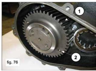
Fasten the ring gear stop (1, fig. 77) using (2) M10x25 screws. Calibrate the screws with a torque wrench as indicated in Section 3, "Screw Tightening Calibration" (1, fig 78).
