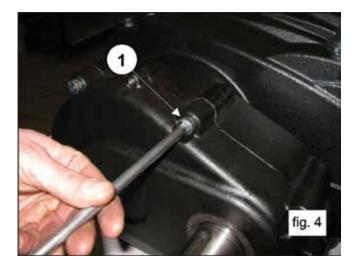
Position the 3 grub screws or M8 threaded screws (1, fig. 5) with the function of extractors in the holes and two sufficiently long M10 screws with the function of supporting the cover (2, fig. 5).
