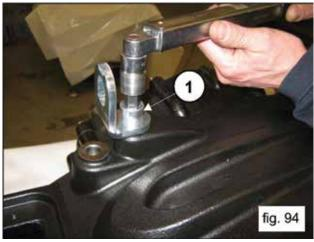
Insert oil in the casing as indicated in the Owner's Manual, Section 7.4.
