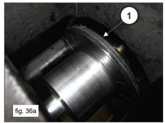
Remove the tool and remove the oil seal (1, fig. 36b).
