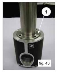
Lock the plunger guide in a vice with the aid of a special tool and calibrate the screws with a torque wrench (1, fig. 44) as indicated in chapter 3 "Screw Tightening Calibration".
