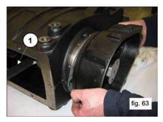
Assemble the reduction gear box (and related seal) using an extractor hammer (1. fig. 64).
