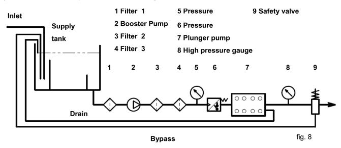
The filters must be installed as close as possible to the pump. They must be easily accessible for inspection amd must have the following specifications:
