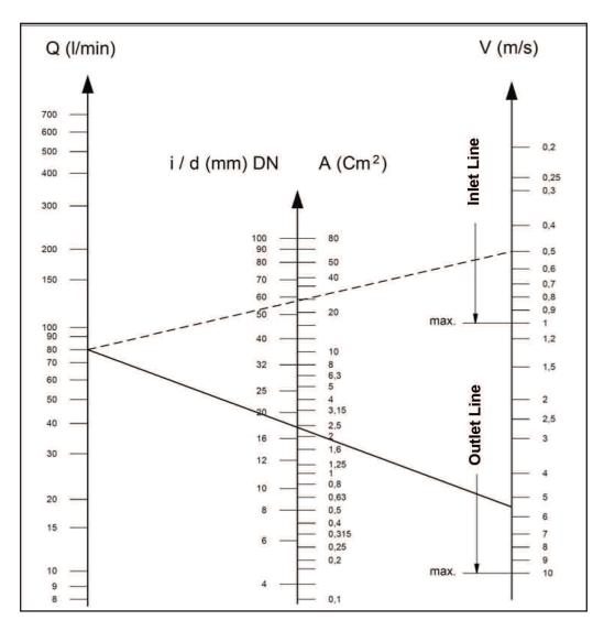
The diagram does not take into account the hose and valve resistance, the pressure drop due to the pipe length, the viscosity and the temperature of the pumped fluid. If necessary, contact our Customer Service Department.
