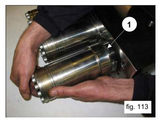
When removing the liners be careful not to lose the valve springs and their flat valves (1 and 2,fig. 114). Because they are only held in position by the surrounding parts, they could easily fall out.
