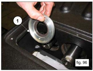
Make sure that the cover completely enters its seat (1, fig. 97), being careful not to damage the lip of the radial seal ring. Screw in the oil seal covers using 2 (M6 x 30 grub screws (1, fig. 98).
