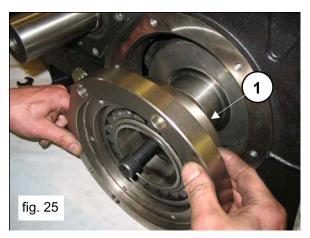
Lay the crankshaft on the bottom of the casing. Separate the bearing support cover from the bearing, using a striking hammer (1, fig. 26).
