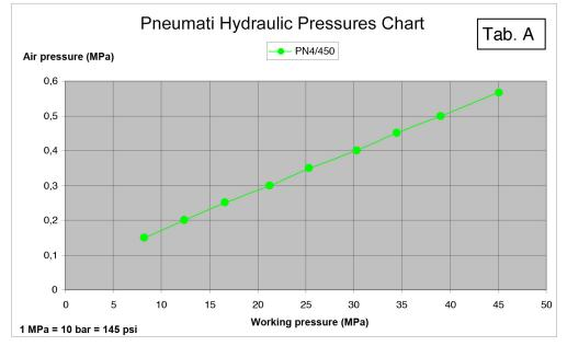
At the pneumatic pressure of 0.58 MPa the air consumption is 28 NI/min.
