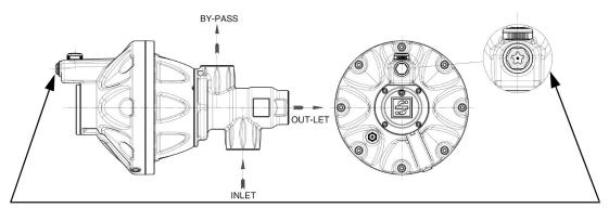
**WARNING:** In horizontal installation, the parts pos. 15 - G3/8 RELIEF PLUG and pos. 17 - G 3/8 OIL PEEPHOLE shall be inverted. **Important:** the tank must always be oriented upwards. Make sure that the oil level is half the peephole.
