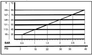
Naturally, if the application allows for feeding the pump with 45 psi (3 bar) even at low temperatures (for example:  $115^{O}F/45^{O}C$  the life of the wet end of the pump will be even longer.
