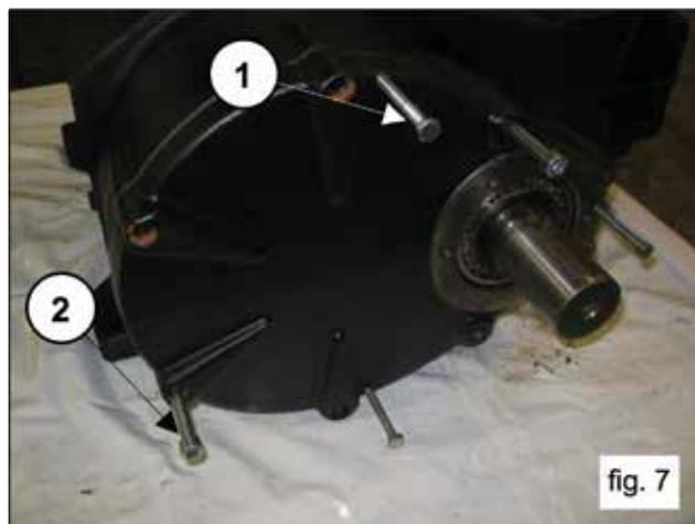
Screw on the 3 threaded screws (1, fig. 8) and simultaneously, using the appropriate tool (p/n F27516700), hammer on the tool itself so that the bearing remains on the pinion when extracting the cover (1, fig. 9).
