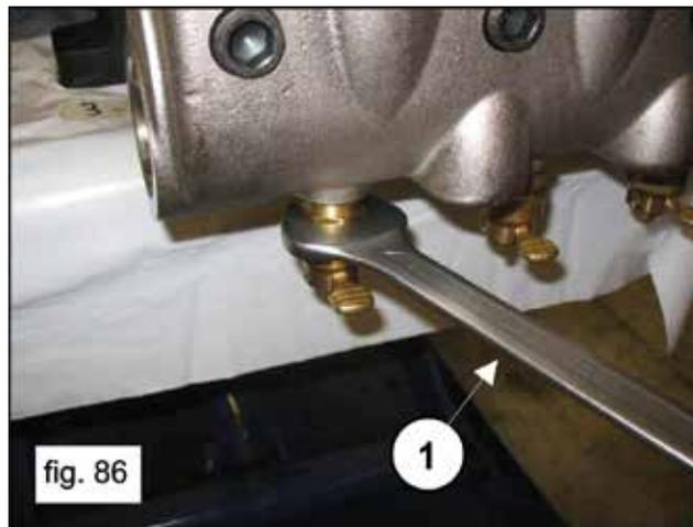
Disassemble the suction and delivery valve units by screwing on an M10 screw long enough to act on the valve and extract the valve guide from the valve seat (1, fig. 87).
