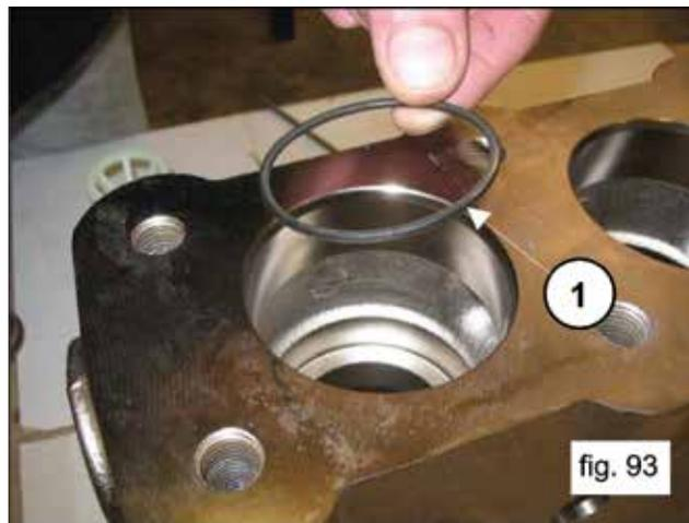
Be sure that the O-ring and the anti-extrusion ring are perfectly fit into their seats. Insert the suction valve unit together with the spacer (1, fig. 94). The valve unit must be fully inserted, as shown in 1, fig. 95.
