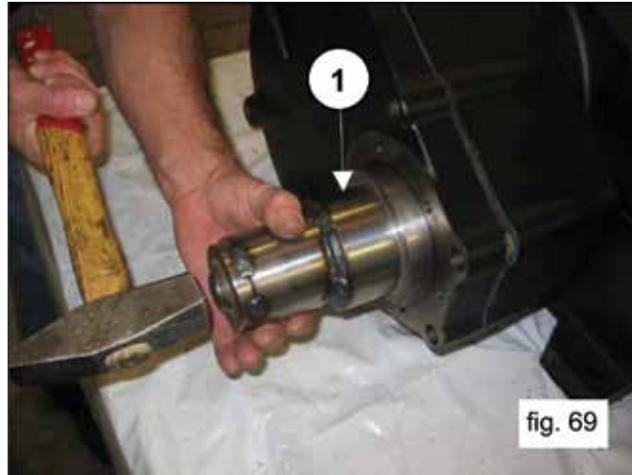
Insert the oil seal inside the reducer flange using the proper tools, p/n F27515900 and F27548200 (1, fig. 70). Before proceeding with oil seal assembly, verify the conditions of the sealing lip. If replacement is necessary, position the new ring as indicated in fig. 71.
