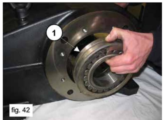
Insert the shaft (1, fig. 29) until the pre-assembled bearing is aligned with the edge of the crankcase (1, fig. 43).
