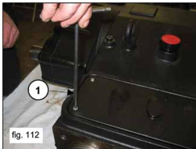
Manually rotate the shaft so that the 3 plungers are in the top dead center position.
