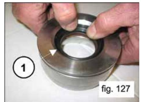
Couple the packing support to the liner (1, fig. 128).
