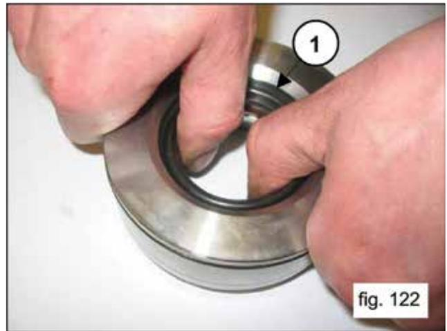
To remove the low pressure packing, use a shim or another tool that doesn't damage the seat of the packing support (1, fig. 123).
