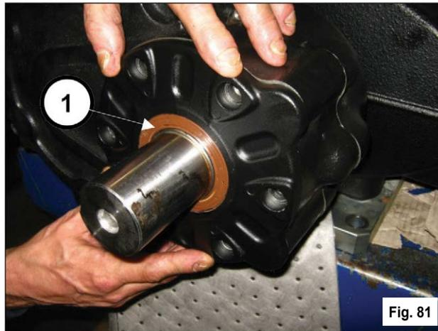
Tighten the 6 M10x25 screws (1, fig. 82). Calibrate the screws with a torque wrench as indicated in chapter 3 SCREW TIGHTENING CALIBRATION.
