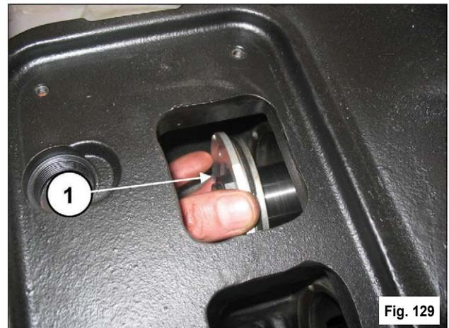
Replace the oil seal (1, fig. 130) and the external O-ring (2, fig. 130).
