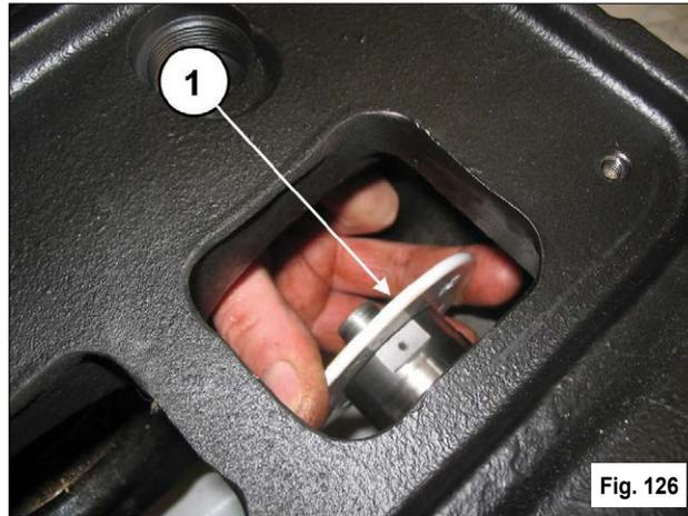
If replacement of the plunger guide oil seal is needed, disassemble the oil seal cover by operating as follows: Unfasten the two screws of the oil seal cover (1, fig. 127).
