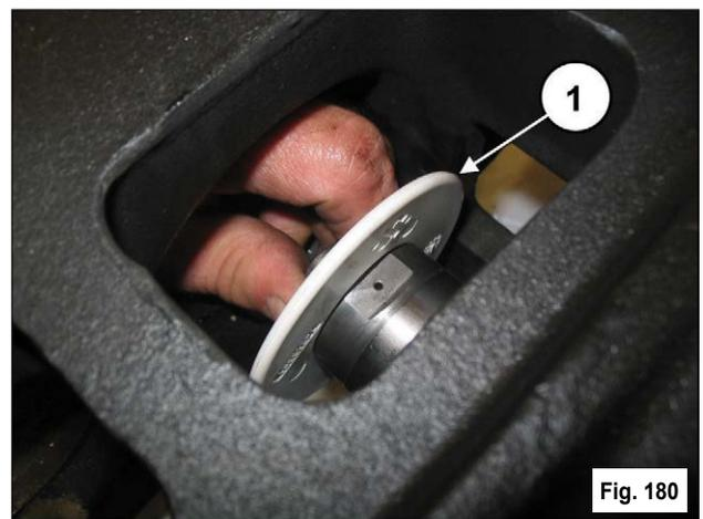
Insert the  $\varnothing 10 \times 18 \times 0.9$  washer in the plunger fixing screw (1, Fig. 181).
