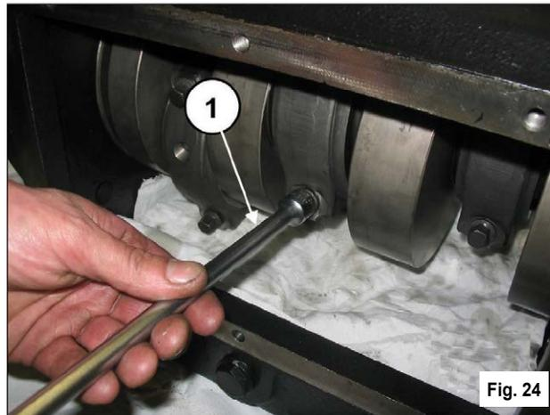
Disassemble the connecting rod caps with the split bearings; be particularly aware of disassembly order.
