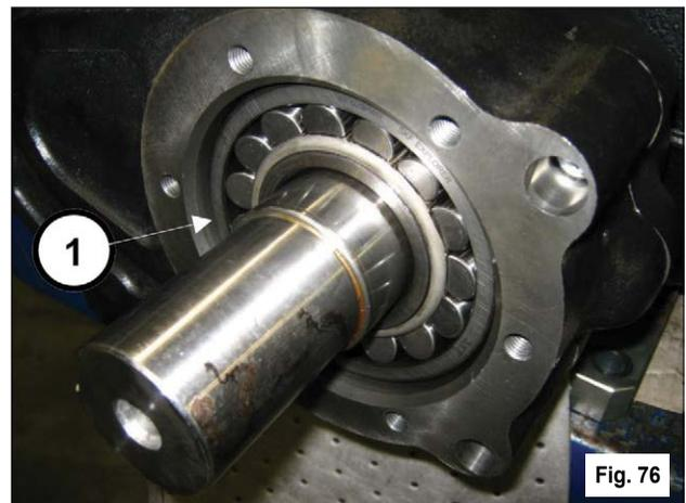
Insert the seal ring inside the pinion cover using the special tool p/n 27548200 (1, Fig. 77).
