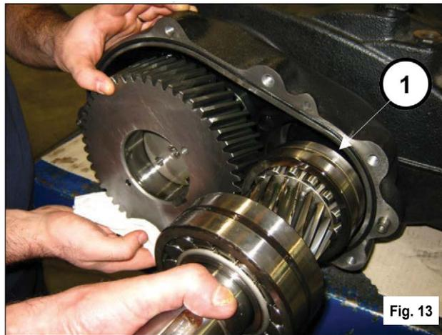
Now it is possible to fully remove the ring gear (1, fig. 14).
