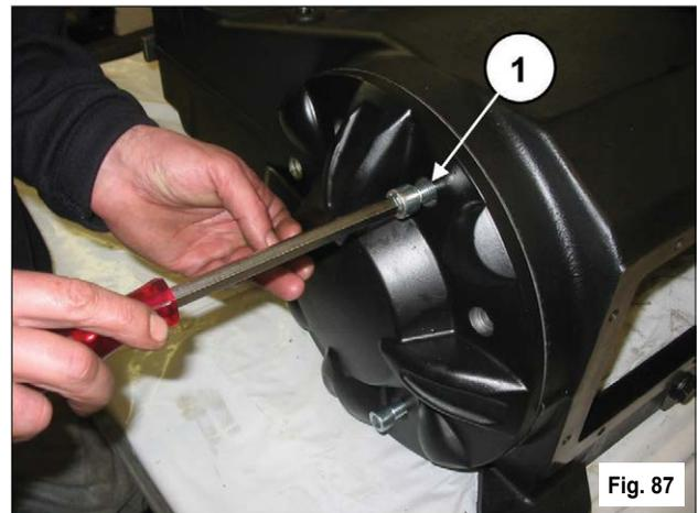
Complete the assembly of the mechanical part by fitting the plugs and lifting eyebolts with the relevant O-rings. Insert oil in the casing as indicated in the owner's manual, par. 7.4.
