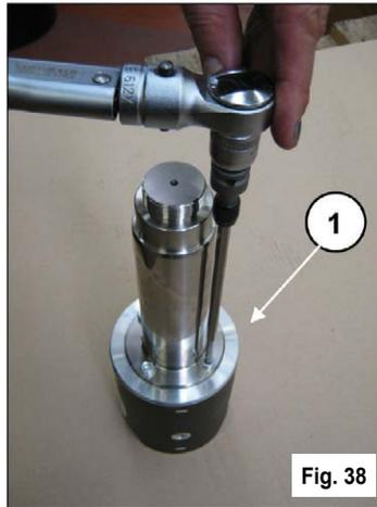
**2.1.2 Crank Mechanism Assembly**
