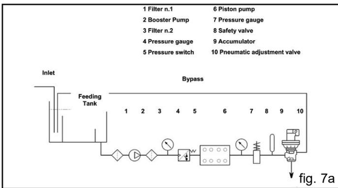
The filter must be installed as close as possible to the pump, should allow easy inspection and have the following characteristics:
