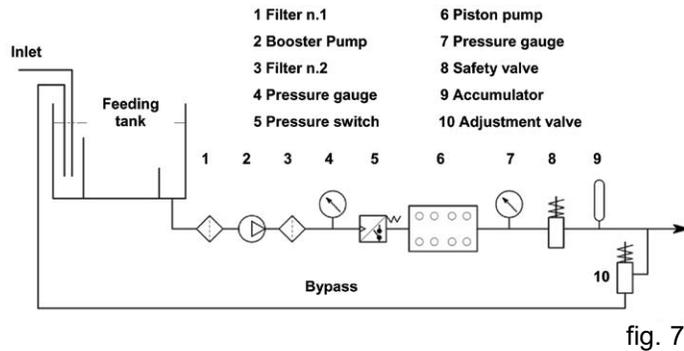
**With the pneumatic adjustment valve:**
