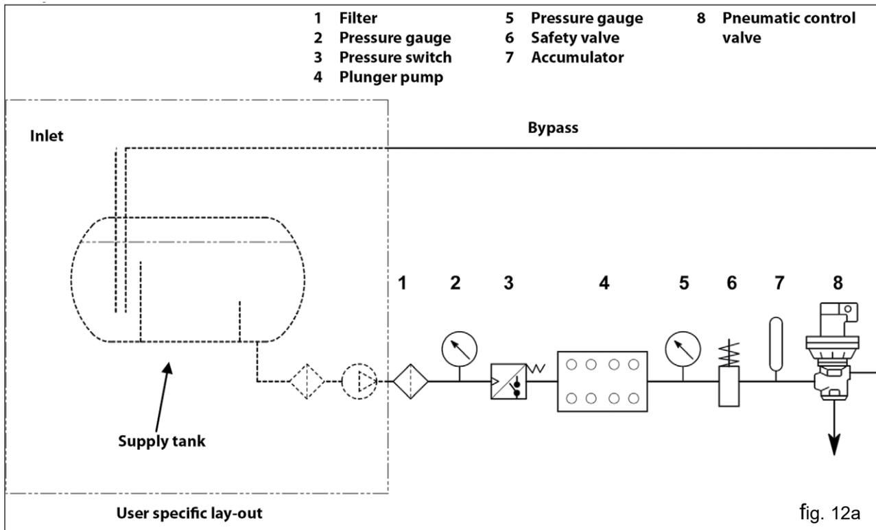
The filter must be installed as close as possible to the pump and be easily inspected.
