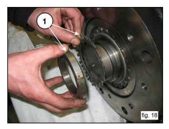
Screw a SKF KM19 type ring nut onto the pressure sleeve (1, fig. 19), then loosen the sleeve using an appropriate wrench (1, fig. 20).
