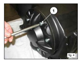
Disassemble the crankcase cover by unfastening the relevant screws (1, fig. 5).
