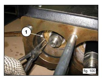
Extract the wiper support. To facilitate the extraction it is possible to use the front holes M5 to apply a threaded rod with extractor hammer (1, fig. 101).
