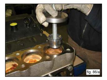
Repeat points D) and E) to extract the valves parts and valves housings from the inlet valve units (fig. 87).
