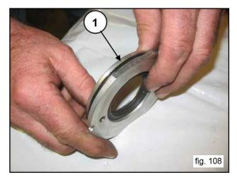
Make sure that the cover completely enters its seat (1, fig. 109) being careful not to damage the lip of the seal ring.
