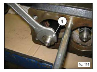
Check and verify the wear condition of the sliding area on the plunger spacer and replace if necessary.
