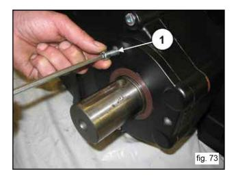
Insert the key  $16 \times 10 \times 90$  in the pinion.
