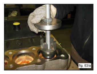
Repeat points D) and E) to extract the balls and valves housing from the intlet valve units (fig. 84).
