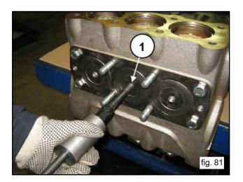
D) Extract the balls using a magnet or other tool (1, fig. 82).
