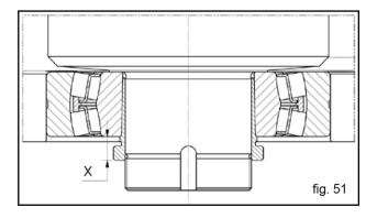
Screw the ring nut and fasten the sleeve until the dimension "X" is reduced by a value ranging between 0.7 and 0.8 mm (fig. 52).
