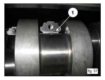
Apply the lower split bearings to the caps, (1, fig. 58) being sure that the split bearings' reference key is positioned in the appropriate seat on the cap (1, fig. 58).
