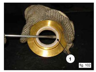
If the plunger guide seal ring needs replacing, the oil seal cover removal is as follows: Unscrew the two screws locking the oil seal cover (1, fig. 103).
