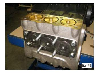
B) Remove the valve plugs by using a M10 extractor hammer (1, fig. 80).
