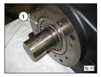
Manually insert the pressure sleeve to maintain the shaft alignment (1, fig. 44).
