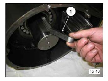
Remove the pinion by using a slide hammer applying it to the M14 hole (1, fig. 14).
