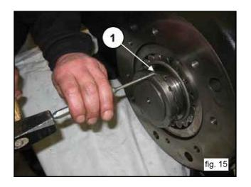
Insert a spacer under the connecting rod to block shaft rotation (1, fig. 16).
