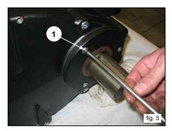
On the opposite side, unfasten the screws (1, fig. 4) and then remove the bearing cover.
