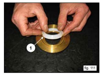
Position the O-ring on the wiper support (1, fig. 112).
