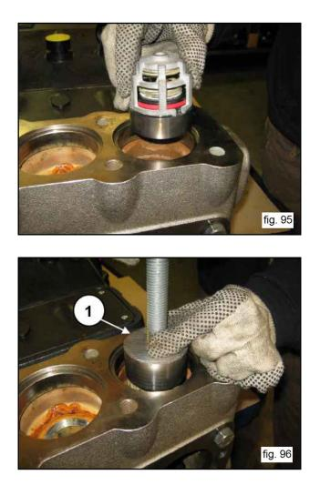
Reassemble the valve caps and, at the front, reposition the valve covers. At the front, calibrate the M16 x 55 screws and M16 nuts with a torque wrench as indicated in chapter 3 "SCREW CALIBRATION".
