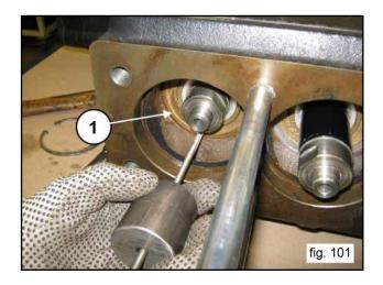
Remove the wiper using a simple tool as indicated in (1, fig. 102), making sure not to damage the housing. If necessary, remove the plunger spacer before removing the wiper support (see par. 2.2.3.1).
