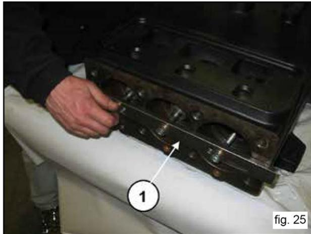
Remove the pressure sleeve (1, fig. 26).
