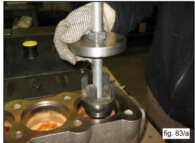
Repeat points D) and E) to extract the balls and valves housing from the inlet valve units (fig. 84).
