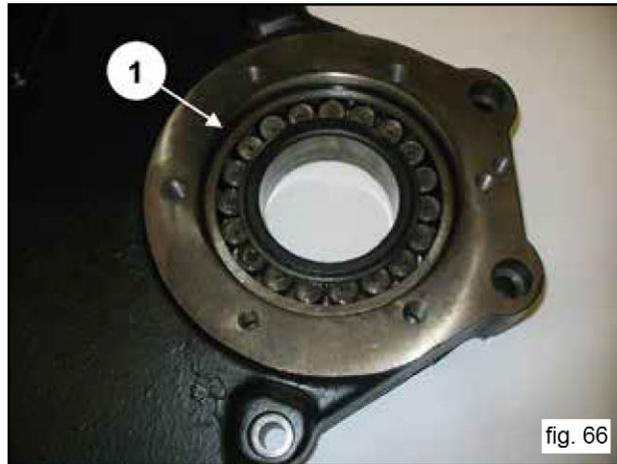
Assemble the reducer cover (1, fig. 67) and fasten it using 8 M10 x 50 screws (1, fig. 68). Use a stopper to avoid the bearing coming out of the seat (1, fig. 69). Calibrate the screws with the torque wrench as indicated in paragraph 3 "SCREW CALIBRATION".
