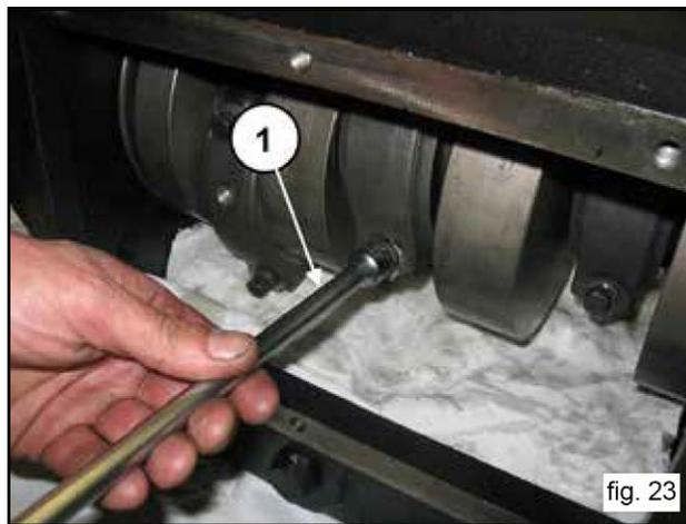
Disassemble the connecting rod caps with the split bearings; be particularly aware of disassembly order.
