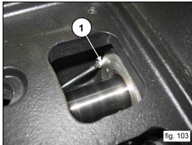
Position the guide plunger at bottom dead center, screw the extractor #F7516400 included the M5 adapter #F27516500 in the holes in the cover (1, fig. 104) and remove the cover from the pump seal through the upper openings for the crankcase (1, fig. 105).
