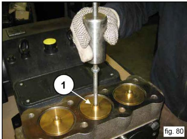
C) Remove front plugs by using a M16 extractor hammer (1, fig. 81).
