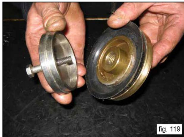
Lubricate the plunger seal with abundant OCILIC 250 silicone grease #F12001600 (fig. 120).
