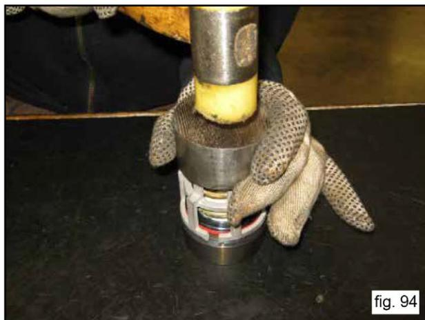
Assemble the inlet and outlet valve units using tool #F27764000, (see mechanical drawing in par. 4.1), ensuring that the tapered surfaces of the seats are locked in the tapered seats present on the head (fig. 95 and fig. 96)
