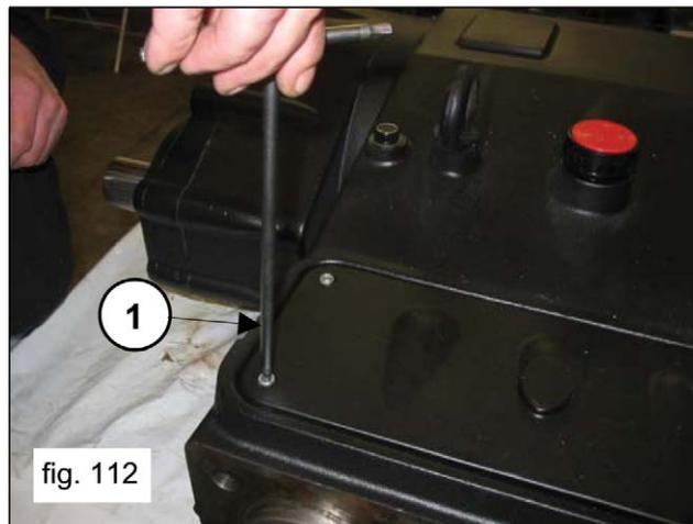
Manually rotate the shaft so that the 3 plungers are in the top dead center position.
