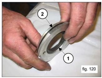
Separate the packing support from the liner (1, fig. 121) to access the pressure packings (1, fig 122).
