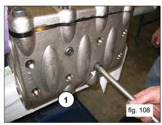
Proceed with calibrating the M16 by 180 screws with the torque wrench as indicated in paragraph 3. "SCREW CALIBRATION"
