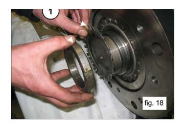
Screw a SKF KM19 type ring nut onto the pressure sleeve (1, fig. 19), then loosen the sleeve using an appropriate wrench (1, fig. 20).
