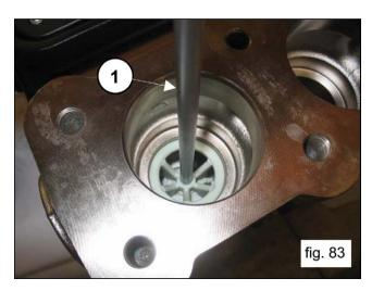
Remove the suction valve unit using a slide hammer applied to the M10 hole of the valve guide (1, fig. 84).
