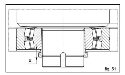
Screw the ring nut and fasten the sleeve until the dimension "X" is reduced by a value ranging between 0.7 and 0.8 mm (fig. 52).
