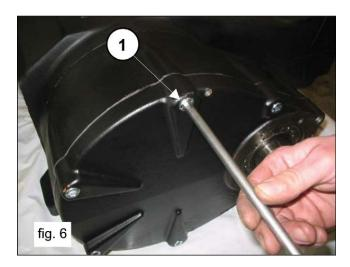
Insert 3 dowels, or 3 M8 threaded screws (1, fig. 7) in the appropriate holes to aid extraction, and two sufficiently long M10 screws in order to support the cover (2, fig. 7).
