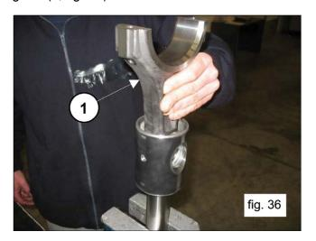
To separate the rod from the plunger guide, unfasten the M10 hexagonal-head screws using a size 17 socket wrench (1, fig. 37).
