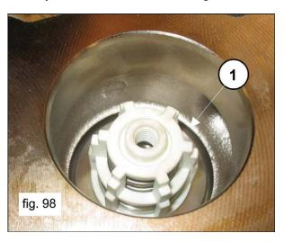
Insert the anti-extrusion ring, exploded view item 16 in Owner's Manual (1, fig. 99).
