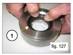
Couple the packing support to the liner (1, fig. 128).
