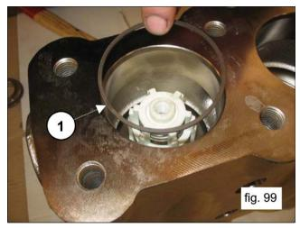
Insert the O-ring, exploded view item 17 in Owner's Manual, (1, fig. 100).
