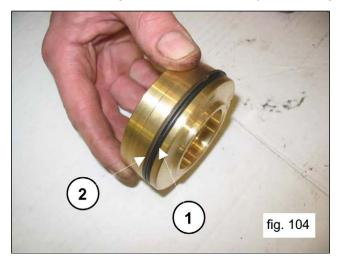
Insert the valve plug complete with O-rings and anti-extrusion ring.
