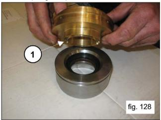
Insert the oil seal in its cover (1, fig. 129) using a stopper p/n 27515800.
