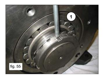
Remove the device that blocks the connecting rods using p/n 27566200 (1, fig. 31).
