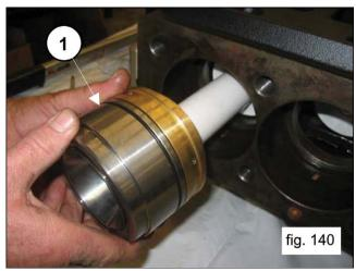
Be sure that the liner-support unit is correctly positioned in its seat (1, fig. 141).
