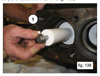
Calibrate the screws using the torque wrench as indicated in paragraph 3. "SCREW CALIBRATION"
