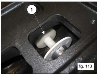
Turning the shaft, move the plunger forward so that the stopper, moving forward itself, can push out the packing support and the entire plunger unit (1, fig. 114).
