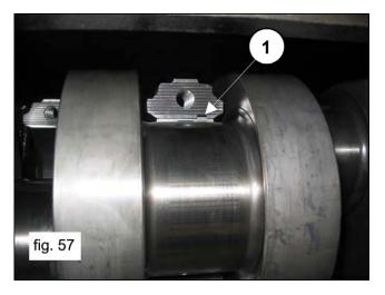
Apply the lower split bearings to the caps, (1, fig. 58) being sure that the split bearings' reference key is positioned in the appropriate seat on the cap (1, fig. 58).
