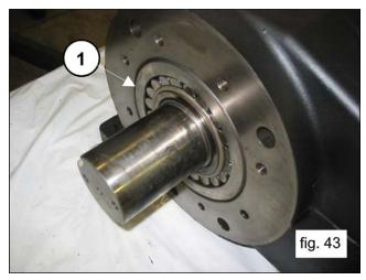
Manually insert the pressure sleeve to maintain the shaft alignment (1, fig. 44).
