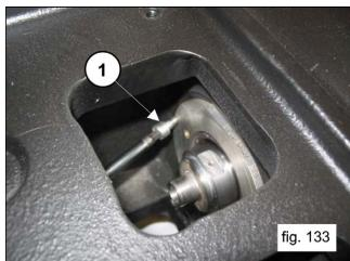
Calibrate the screws using a torque wrench as indicated in paragraph 3. "SCREW CALIBRATION"
