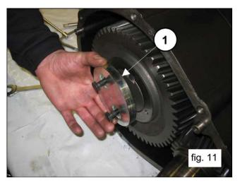
Remove the ring gear (1, fig. 12). If necessary, use a slide hammer applying it to the 2 M8 holes (2, fig. 12).
