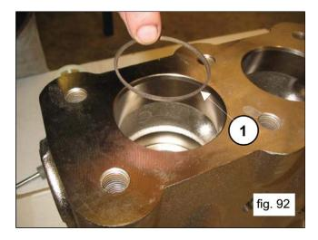
Insert the O-ring, exploded view item 5 from Owner's Manual (1, fig. 93).
