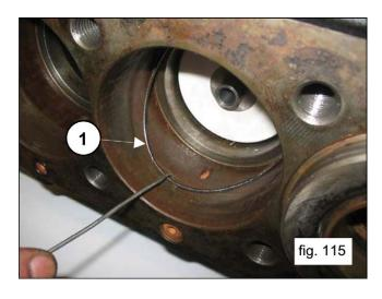
Remove the wiper rings from the plunger guides (1, fig. 116).
