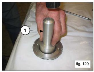
Position the O-ring (1, fig. 130) in its seat on the oil seal cover, and insert the assembled unit inside the
