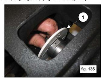
Insert the 14 x 2 O-ring in its correct seat on the plunger bolt (1, fig. 136).
