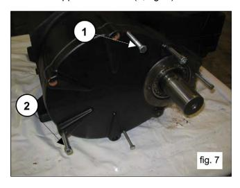
Screw on the 3 threaded screws (1, fig. 8) and simultaneously, using the appropriate tool (p/n 27516700), hammer on the tool itself so that the bearing remains on the pinion when extracting the cover (1, fig. 9).
