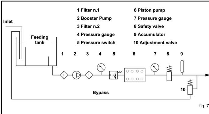
**With the pneumatic adjustment valve:**
