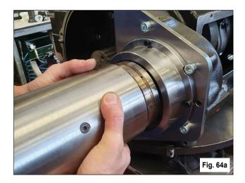
Position the bearing to the end stroke (1, fig. 65)
