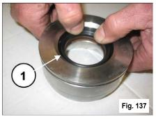
Couple the packing support to the liner (1, fig. 138).
