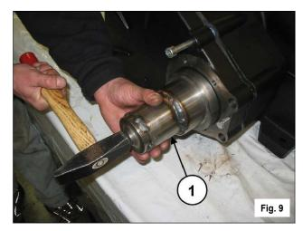
When this operation is complete, remove the reducer cover and then slip off the bearing from the pinion. Remove the screws that fasten the ring gear stopper (1, fig. 10), and remove the stopper itself (1, fig. 11).
