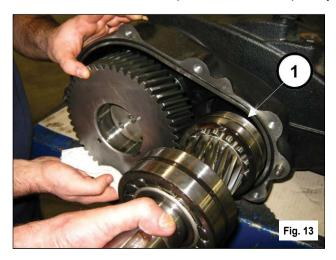
Now it is possible to fully remove the ring gear (1, fig. 14).
