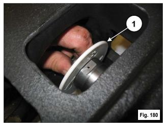
Insert the Ø10x18x0.9 washer in the plunger fixing screw (1, Fig. 181).
