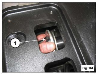
Replace the oil seal (1, Fig. 165) and the external O-ring (1, Fig. 165).
