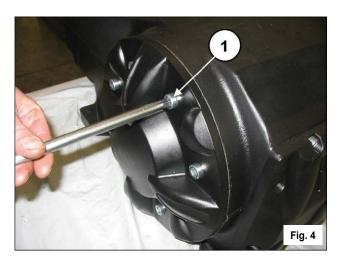
Disassemble the crankcase cover by unfastening the relevant screws (1, fig. 5).
