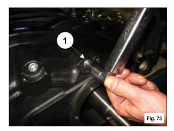
Insert the 60x130x46 bearing on the pinion (1, Fig. 74).
