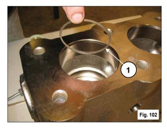
Insert the O-ring, exploded view item 5 from Owner's Manual (1, fig. 103).
