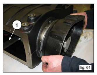
Assemble the reduction gear box (and relative seal) using an extractor hammer (1, fig. 62).
