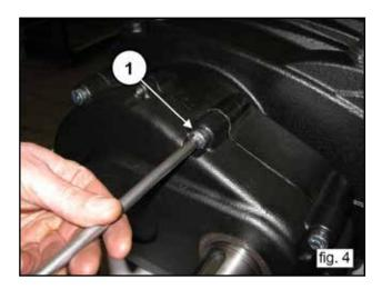
Position the 3 grub screws or M8 threaded screws (1, fig. 5) with the fuction of extractors in the holes and two sufficiently long M10 screws with the function of supporting the cover (2, fig. 5).
