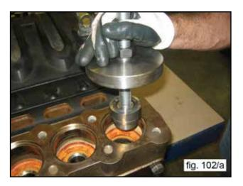
Repeat points D) and E) to extract the valves parts and valves housings from the suction valve units (fig. 103).
