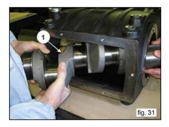
In the event that it is necessary to replace one or more con-rod or plunger guides, operate as follows: Unscrew the screws with tool code (#F27566200) to unlock the con-rods (1, fig. 32) and then exctract the con-rod plunger guides units from the crankcase rear opening (1, fig. 33).
