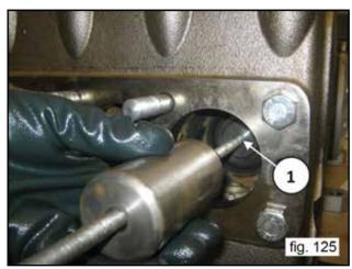
Using a M16 cover screw, tighten using a T-handle wrench on the seal support so that it acts as an extractor (1, fig. 126), once the seat has come out, extract the pack, consisting of the support and the plunger seal (1, fig. 126/a).
