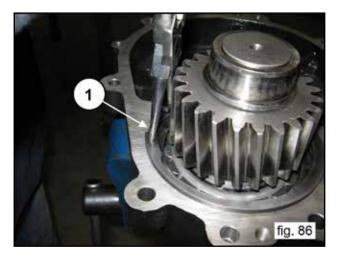
Assemble the reduction gear cover with the aid of an extractor hammer (1, fig. 87) and fasten it with 7 M10x40 screws (1, fig. 88). Make sure to properly couple the two components on the bearing 40x90x23. Calibrate the screws with a torque wrench as indicated in chapter 3 "SCREW CALIBRATION".
