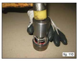
Assemble the inlet and outlet valve units using the buffer #F27812000, (see mechanical drawing in par. 4.1), ensuring that the tapered surfaces of said seat are locked in the tapered seats present on the head (fig. 111 and fig. 112).
