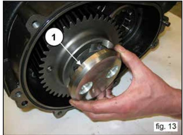
Remove the ring gear (1, fig. 14). If necessary, it is possible to use an extractor hammer to be applied on the 2 M8 holes (2, fig. 14).
