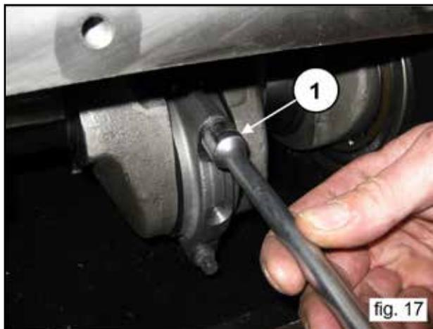
Remove the con-rod caps with the lower semi-bearings, taking special care of the disassembly sequences during disassembly.
