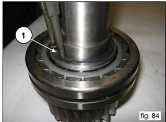
Insert the pinion pre-assembled inside its housing in the reduction gear cover, with the aid of an extractor hammer (1, fig. 85).
