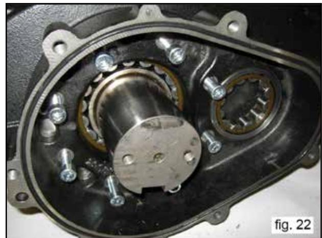
Position the 3 grub screws or M8 threaded screws (1, fig. 23) with the function of extractors in the holes and two sufficiently long M10 screws with the function of supporting the reduction gear box (1, fig. 23).
