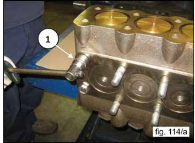
Remove the head from the pump crankcase (1, fig. 115).
