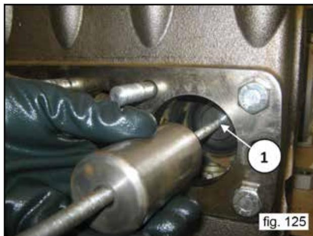
Using a M16 cover screw, tighten using a T-handle wrench on the seal support so that it acts as an extractor (1, fig. 126), once the seat has come out, extract the pack, consisting of the support and the plunger seal (1, fig. 126/a).
