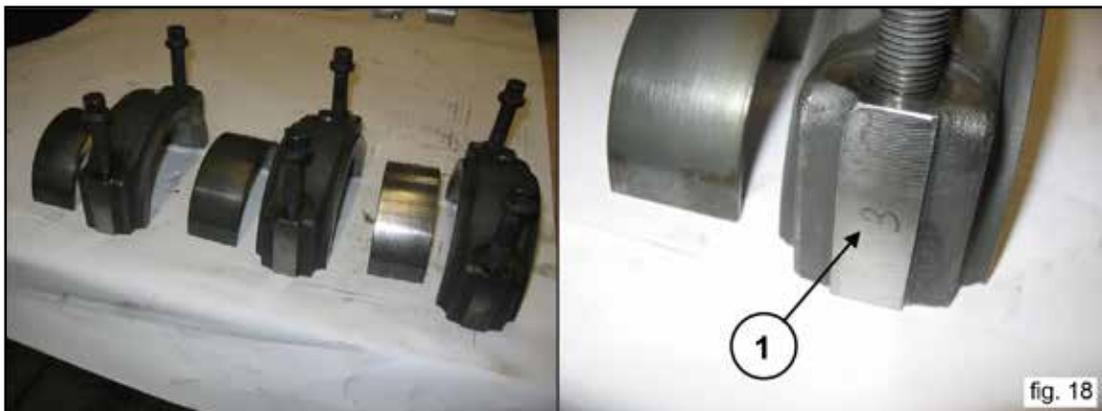
Advance the con-rods completely in the direction of the hydraulic part to allow extraction of the crankshaft. To facilitate this operation, use special tool (#F27566200), (1, fig. 19).
