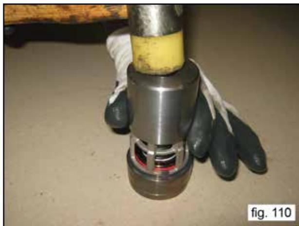
Assemble the inlet and outlet valve units using the buffer #F27812000, (see mechanical drawing in par. 4.1), ensuring that the tapered surfaces of said seat are locked in the tapered seats present on the head (fig. 111 and fig. 112).
