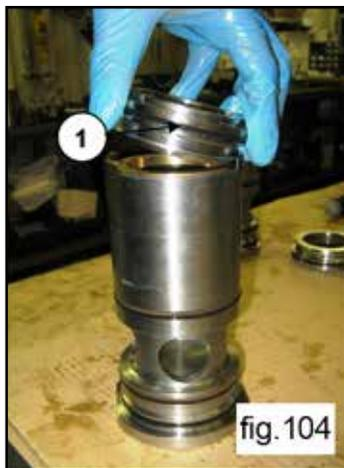
Remove the high and low pressure seals from their seats (1, fig. 105 and 106).
