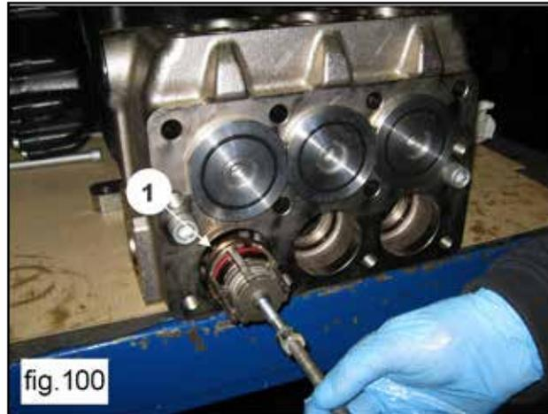
Unscrew the valve opening device by means of a 30 mm spanner (1, fig. 101)
