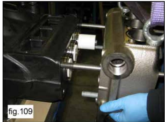
Remove the 3 manifold locating bushes from the casing.
