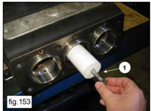
Calibrate the screws with a torque wrench as indicated in paragraph 3 "Screw Tightening Calibration".
