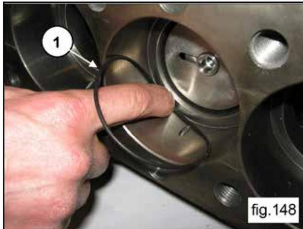
Remove the spray rings from the piston guide (1, fig. 149).
