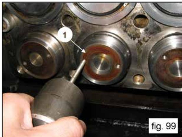
Extract the suction valve unit with the use of a slap hammer(#27516400) to be applied on the M10 hole of the valve guide (1, fig. 100).
