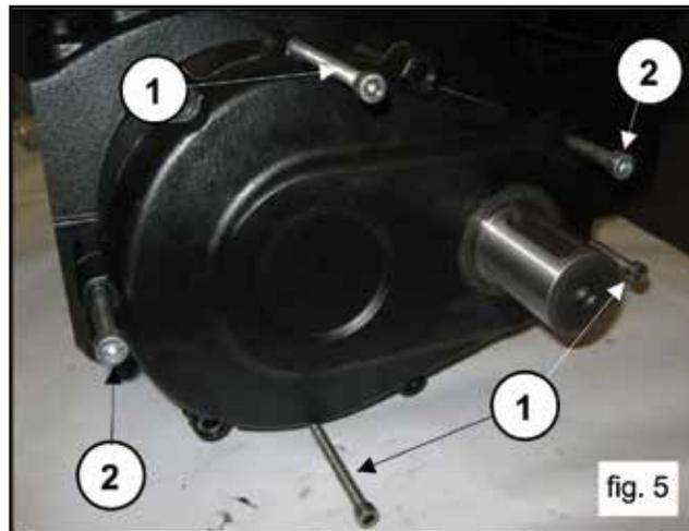
Slowly screw in the 3 M8 screws (1, fig. 6) with the function of extractors to fully remove the cover unit and pinion.
