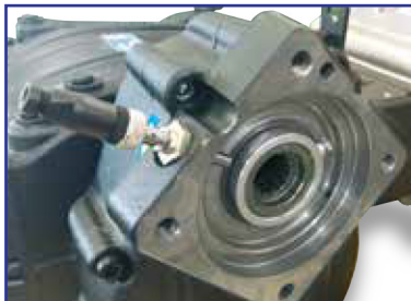
SAE J744-C Spline Shaft 14T 12/24 DP Hydraulic Motor Mount
