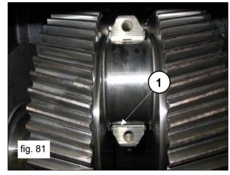
Apply the lower half-bearings to the small ends (pos. 1, fig. 82), making sure that the lugs on the half-bearings are positioned in the slots on the small ends (pos. 1, fig. 82)
