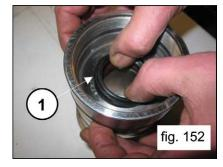
Place the O-ring for the gasket support on its seat (pos. 1, fig. 153).
