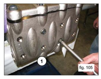
Unscrew and remove the 8 M16X55 screws of the valve cover (pos. 1, fig. 106) and remove the cover (pos. 1, fig. 107).
