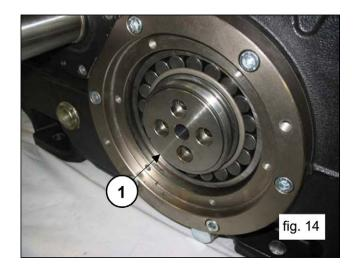
On one side, screw a ferrule (type SKF KM20) onto the pressure bushing (pos. 1, fig. 15), and then unblock the bushing using a striking hammer (pos. 1, fig 16), but do not remove it. Repeat the operation on the other side.
