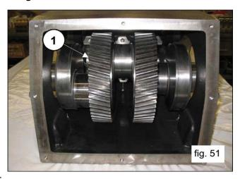
Pre-assemble the PTO shaft:
