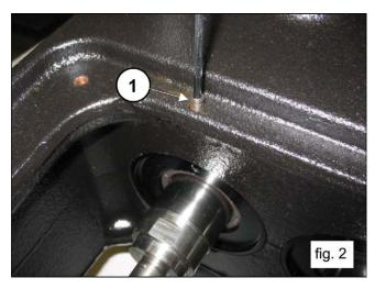
Screw in a threaded bar or an extractor M6 screw in the holes in the oil seal covers (pos. 1, fig.3) and remove the covers from the pump assembly (pos. 1, fig. 4).
