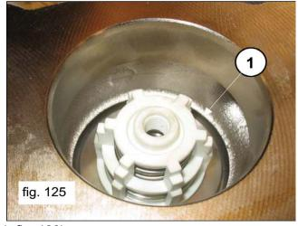
Insert the anti-extrusion ring, exploded position #16 (pos. 1, fig. 126).
