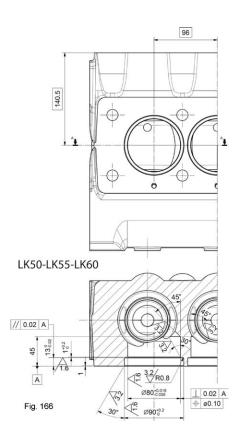
The manifold bushing must be assembled by driving bushes (pos.1) together with the anti-extrusion rings (pos. 2) and O-rings (pos. 3) and shown in fig. 167 for LK36-40-45 and fig. 168 for LK50-55-60.
