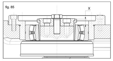
Screw in the M16 screw until there is a reduction in the distance X of between 0.7 mm and 0.8 mm (fig. 86).
