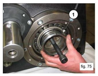
Insert the pressure bushing completely onto the crankshaft (pos. 1, fig. 76 and fig. 77) using a mallet or striking hammer and a pad.
