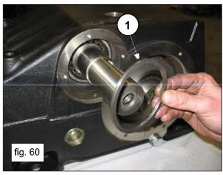
Insert the internal ring (pos. 1, fig. 61) and external ring (pos. 1, fig. 62) of a bearing from one side of the pump only.
