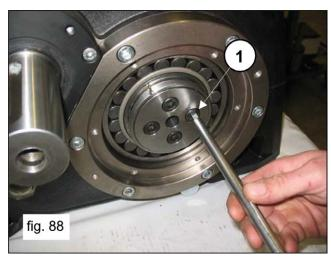
Remove the anti-rotation shim from under the shank of the central connecting rod.
