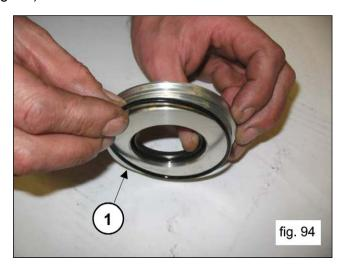
Insert the assembly into the casing and into the seat provided, making sure that the cover completely enters its seat (pos. 1, fig. 95), being careful not to damage the lip of the radial seal ring. Screw in the oil seal covers using 2 M6X30 grub screws (pos. 1, fig. 96).
