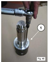
Complete the disassembly of the mechanical parts by removing the oil level lights and the eyebolts.
