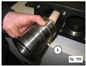
Make sure that the liner/support block goes all the way in and is correctly positioned on its seat (pos. 1, fig. 160).
