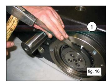
Remove the shim from under the shank of the central connecting rod.
