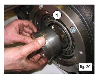
Separate the bushing locking flange from the pressure bushing (pos. 1, fig. 21).
