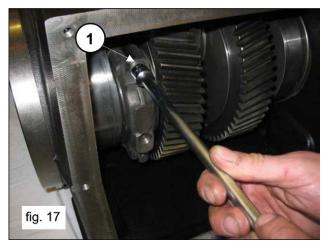
Dismantle the small ends of the connecting rods with the half-bearings. During the operation take particular care to note the order in which the parts are removed
