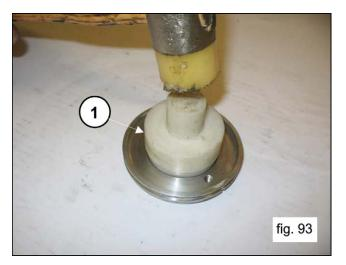
Position the O-ring (pos. 1, fig. 94) on the seat of the oil seat cover.
