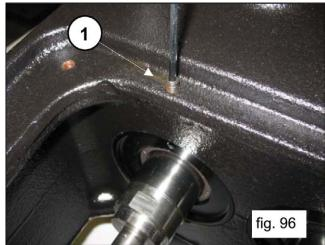
Tighten the screws with a torque wrench as shown in section 3, "Screw Tightening Settings".
