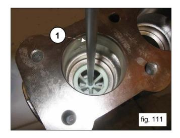
Remove the inlet valve assembly by using a slide hammer puller applied to the M10 hole in the valve holder
