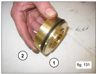
Insert the valve plug, complete with O-ring and anti-extrusion ring. After insertion of the valve assemblies and the valve plugs is complete, replace the valve cover (pos. 1, fig. 132) and screw in the 8 M16X55 screws (pos. 1, fig. 133).
