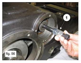
From the side of the casing where the PTO shaft was inserted, proceed to insert the bearing lubrication bushing (pos. 1, fig. 57) and an external bearing ring (pos. 1, fig. 58) using a pad and a mallet or striking hammer.
