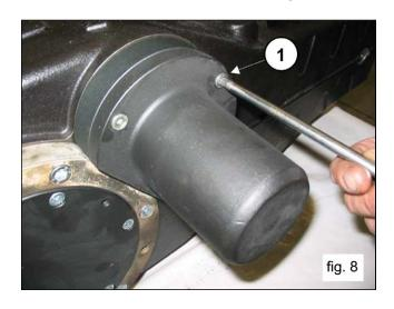
Unscrew the crankcase cover attachment screws (pos. 1, fig. 9) and remove it. Slip off the O-ring and replace it if necessary.
