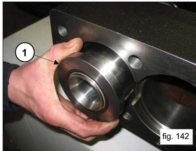
Remove the gasket support assembly and the plastic buffer.
