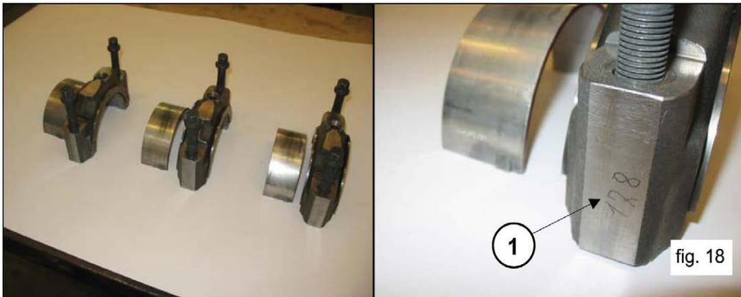
Advance the three big end halves as far as possible in the direction of the head. Slip off the three upper half-bearings of the beg end halves (pos. 1, fig 19).
