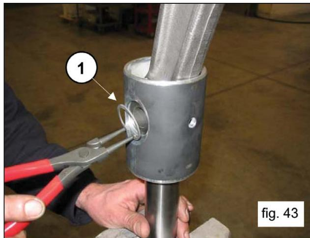
Slip out the pin (pos. 1, fig 44) and take out the connecting rod (pos. 1, fig. 45).
