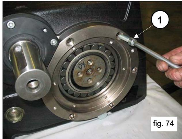
Partly insert the two pressure bushings, keeping the crankshaft lifted up by means of the previously mounted M16 pin (pos. 1, fig. 75).
