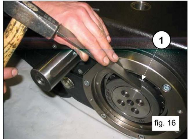
Remove the shim from under the shank of the central connecting rod.
