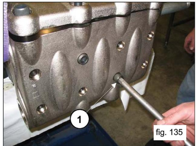
Proceed to tighten the M16X150 screws with a torque wrench, as shown in section 3 “Screw Tightening Settings”.
