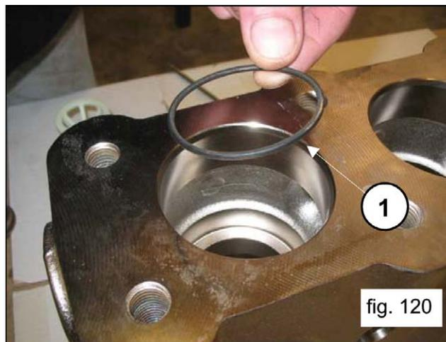
Make sure the O-ring and anti-extrusion ring are perfectly seated in place. Insert the inlet valve assembly (pos. 1, fig 121). The complete valve assembly must be inserted all the way in, as shown in pos. 1, fig. 122.
