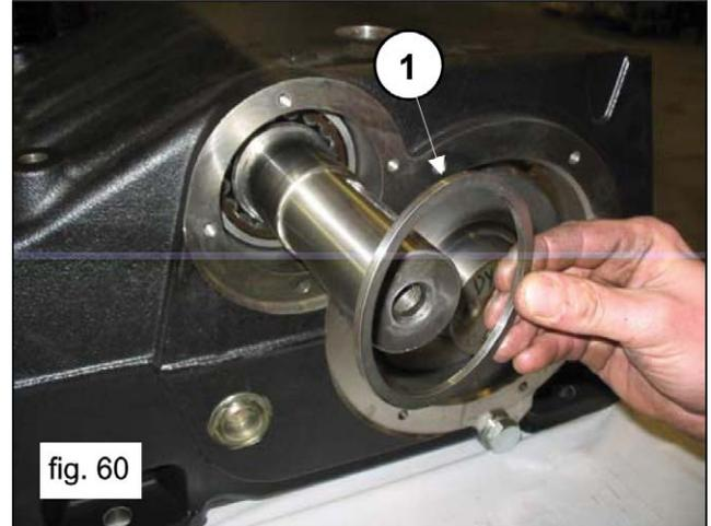
Insert the internal ring (pos. 1, fig. 61) and external ring (pos. 1, fig. 62) of a bearing from one side of the pump only.
