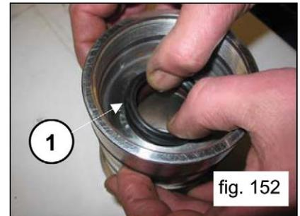
Place the O-ring for the gasket support on its seat (pos. 1, fig. 153).
