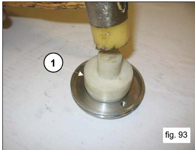
Position the O-ring (pos. 1, fig. 94) on the seat of the oil seal cover.
