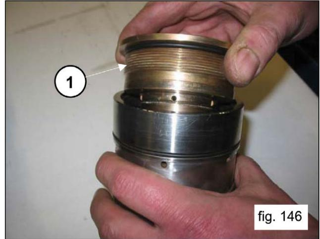
Manually remove the head rings, the pressure gaskets and the restop rings (pos. 1, fig. 147).
