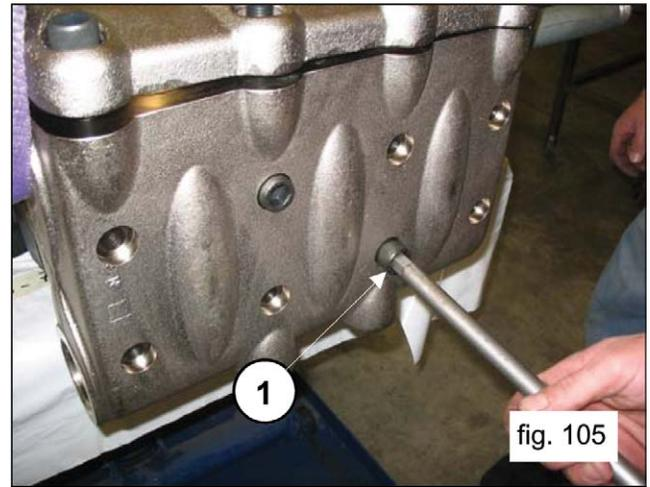
Unscrew and remove the 8 M16X55 screws of the valve cover (pos. 1, fig. 106) and remove the cover (pos. 1, fig. 107).
