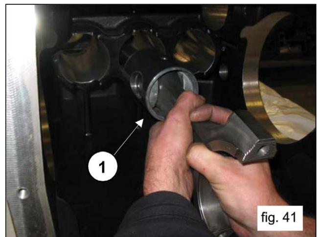
Couple the big end halves to the small ends that were previously dismantled, with reference to their numbering scheme (pos. 1, fig. 42).
