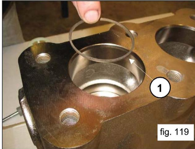
Insert the O-ring, exploded position #5, from Owner's Manual, (pos. 1, fig. 120).
