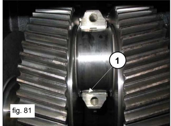
Apply the lower half-bearings to the small ends (pos. 1, fig. 82), making sure that the lugs on the half-bearings are positioned in the slots on the small ends (pos. 1, fig. 82)
