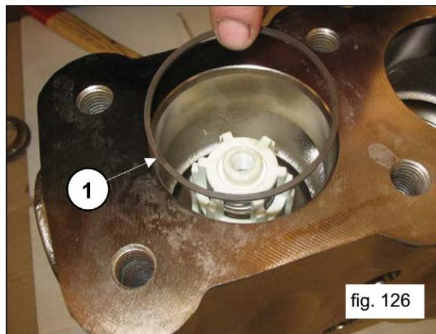
Insert the O-ring, exploded position #17 (pos. 1, fig. 127)
