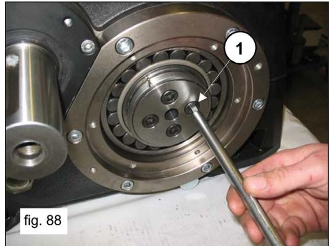
Remove the anti-rotation shim from under the shank of the central connecting rod.
