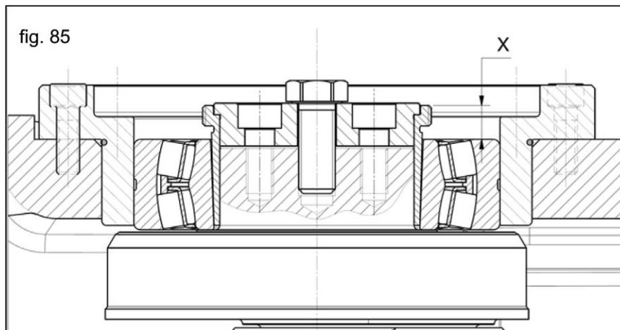
Screw in the M16 screw until there is a reduction in the distance X of between 0.7 mm and 0.8 mm (fig. 86).
