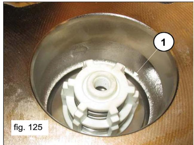
Insert the anti-extrusion ring, exploded position #16 (pos. 1, fig. 126).
