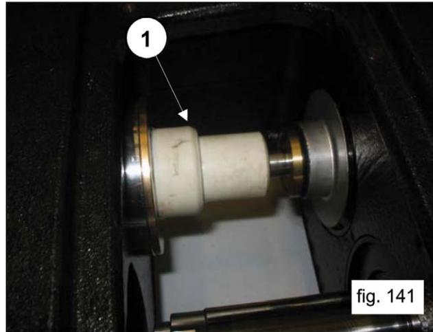
By rotating the shaft, advance the plunger head so that the plastic buffer advances in its turn and expels the gasket support and the entire plunger assembly (pos. 1, fig. 142).
