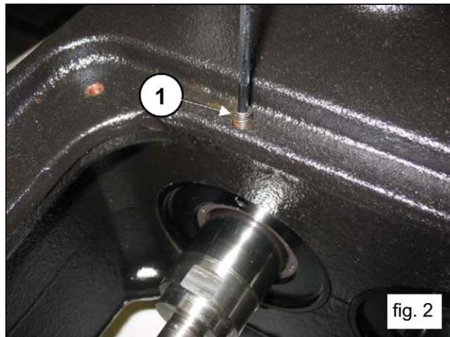
Screw in a threaded bar or an extractor M6 screw in the holes in the oil seal covers (pos. 1, fig.3) and remove the covers from the pump assembly (pos. 1, fig. 4).
