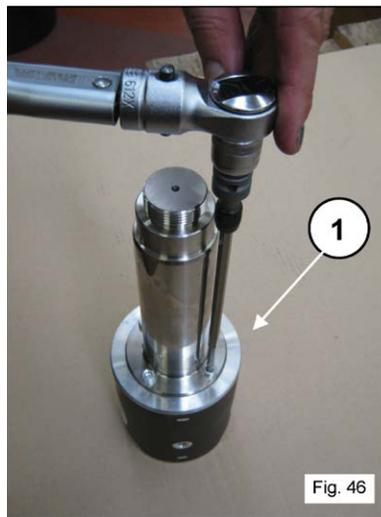
Complete the disassembly of the mechanical parts by removing the oil level lights and the eyebolts.
