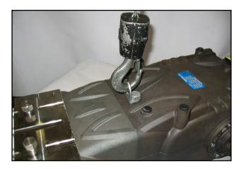
Should it be necessary to disassemble it, to avoid the entrance of dirt in the front part of the casing, close the threaded hole with the cap provided.
