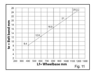
Conclusion: with a wheelbase of 15.75 in (400 mm) and with a dynamometer, loading the belt branch with 16.86 lbs (75 N) as indicated in fig. 12 a "te" bend of approximately .33 in (8.4 mm) is obtained.
