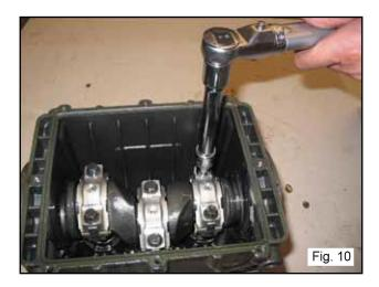
• After having completed tightening operations, check that the con-rod head has a side clearance in both directions.
