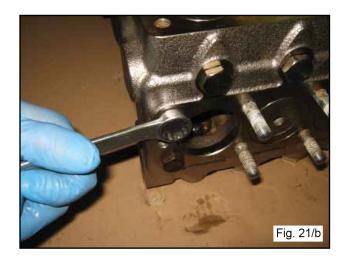
B) Remove the head and the head spacer from the pump casting.
