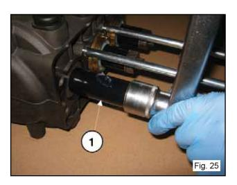
B) Check and verify their conditions, replace if necessary. Check and verify the conditions of the bushes assembled on the spacer (1, fig. 25); replace them if necessary.
