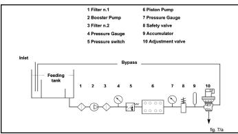
The filter must be installed as close as possible to the pump, should allow easy inspection and have the following characteristics:
