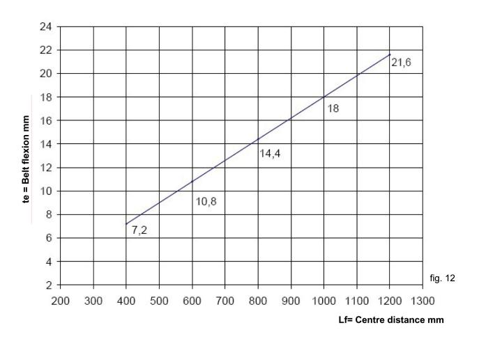
Conclusion: using a dynamometer, by loading the belt with 75 N as indicated in fig. 13, you will obtain a flexion value "te" of about 10.8 mm.
