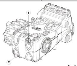
Check the oil level dipstick (pos. 3); refill if necessary. Correct oil level inspection is done with the pump at room temperature; oil is changed with the pump at working temperature by removing the plug (pos. 2), fig 3. Oil inspection and changing is to be carried out as indicated in Section 11.
