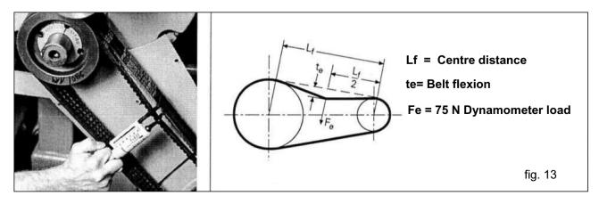
**Note 1.** If not differently indicated by the belt Manufacturer, the inspection of the correct tension value, and the related tension adjustment if needed, is to be carried out after at least 30 minutes of operation in order to obtain belt settling. The best efficiency and maximum duration is obtained with the correct tension value.
