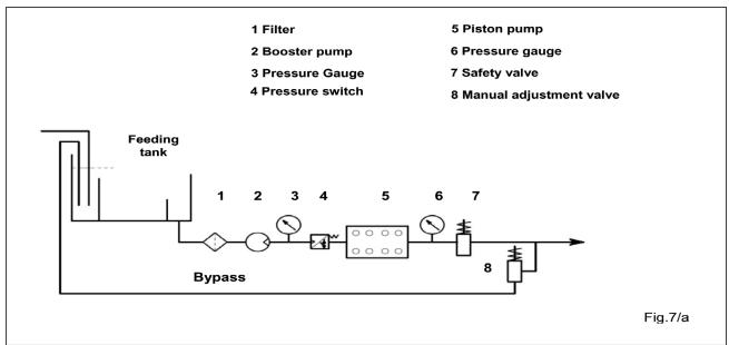
The filter must be installed as close as possible to the pump, should allow easy inspection and have the following characteristics:
