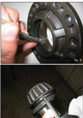
The new roller bearing can be mounted at room temperature with a press or fly press; it is necessary to lay them on the lateral side of the relevant ring nuts with correct rings. The driving operation can be facilitated by heating the relevant parts at a temperature ranging between 250°-300°F (120°-150°C), making sure that the ring nuts are correctly fitted into their seats.
