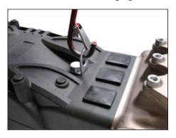
In case of disassembly, to avoid letting dirt inside the front part of the crankcase, close the threaded hole with the supplied cap.
