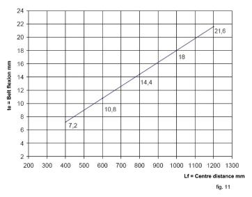
Finally, given a distance between pulley centers of 600 mm and a load of 75 Nm a belt flexion "te" of around 10.8 will confirm the correct belt tension as shown in fig. 12.
