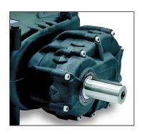
KF pumps can be supplied with a optional gearbox available in 3 different ratios. The gearbox can be mounted on the left or right side of pump in 4 different angles. Ratios R=1.25:1-R=1.50:1-R=1.83:1
