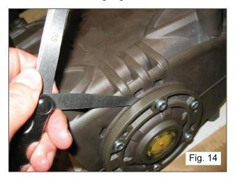
Determine the shim pack, using the table below:
