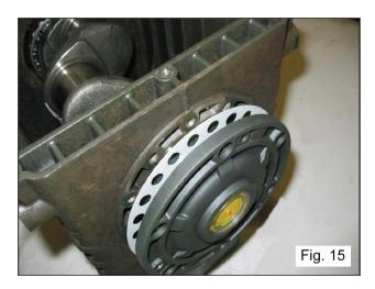
Once the type and number of shims have been determined using the table, check the following: assemble the shim pack on the indicator side cover centering (fig. 15), secure the cover to the crankcase, following the procedure in par. 2.1.2 and tighten the screws to their recommended torque.
