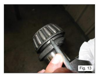
The new roller bearing can be mounted at room temperature with a press or fly press; it is necessary to lay them on the lateral side of the relevant ring nuts with appropriate rings. The driving operation can be facilitated by heating the relevant parts at a temperature ranging between 250°-300° F(120°-150° C), making sure that the ring nuts are correctly fitted into their seats
