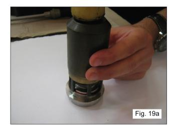
Insert the inlet and outlet valve units, checking that they are fully inserted in the head seat. Then apply the valve cover and calibrate the respective M12 x 35 screws at the required tightening torque.
