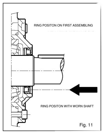
Note: Should the shaft show diameter wear where there is the seal lip, it is possible to avoid grinding by fitting the seal further as indicated in Fig. 11. Before installing the cover (sight glass side) check that the shim rings have been placed. To help the covers fit on the crankcase, you can use 3 screws M6 x 40, and then finish screwing them with the original bolts M16 x 16.
