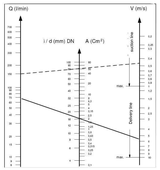
The diagram does not take into consideration the pipe and valve resistance, drop in pressure, due to the pipe length, the viscosity of the pumped fluid, its temperature, etc.
