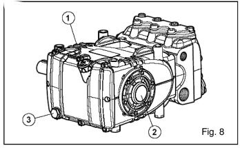
If necessary add the missing oil through the oil plug (1 Fig. 8). Check oil level when the pump is at room temperature. When changing the oil (removing plug 3, Fig. 8), the pump should be at its working temperature.
