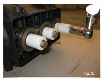
A) Loosen and remove the plunger screw (1, Fig. 25).
