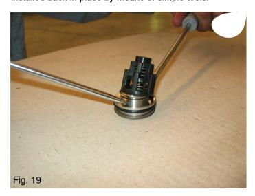
Check the components for wear and replace if necessary. Replace all o-rings of the valve units and plugs, at each inspection.
