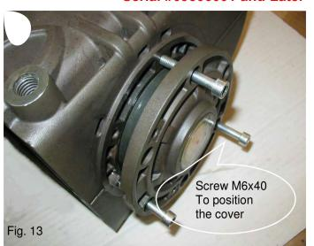
The rolling couple of the crankshaft (with connecting rods coupled) must not exceed 8 Nm.
