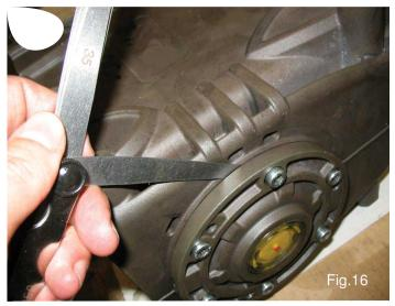
By means of a thickness gauge (see Fig. 16) determine the shim set as indicated in the table below.
