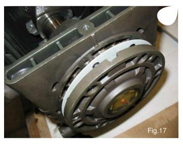
F) If the torque is correct, connect the rods to the crankshaft, otherwise, calculate the shims again as per point "C".
