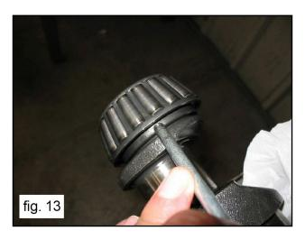
The new bearings can be mounted cold with a press or rocker, supporting it on the lateral surface of the ring nuts involved in press fitting with the rings. The press fitting operation can be assisted by heating the involved parts to a temperature between 250°F - 300°F (120°C - 150°C), ensuring that the ring nuts fit fully into their seats.
