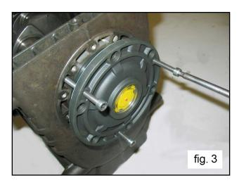
• Push the plunger guides forward with their con-rods to facilitate side extraction of the pump shaft. There are two reference points visible on the crankshaft (indicated with pos. 1 in fig. 4 and in fig. 4/a). These must be turned towards the operator to facilitate extraction.
