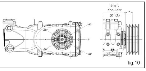
C) Pull the belts according to manufacturer instructions. Excessive pulling can cause reduced bearing life and wear out the pulley prematurely. Pulling depends on different variables as indicated in paragraph 9.12.
