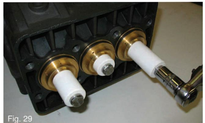
**When disassembling the pumping unit, the O-rings should always be replaced.**
