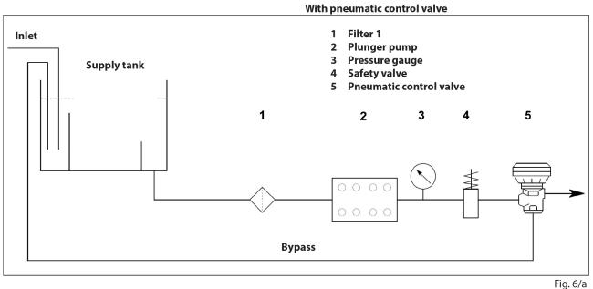
All pumps require a suitable filter. The filter should be installed as close as possible to the pump, should allow easy inspection and have the following characteristics:
