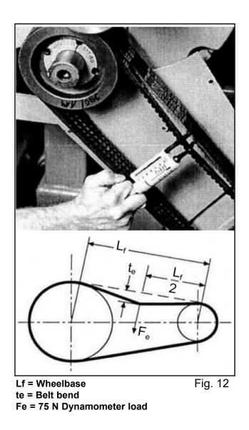
**Note 1** • Unless otherwise stated by the supplier of the belts, control of proper pull and its relative re-tensioning should be performed after no less than 30 minutes of motion necessary for the normal adjustment of the belts. Best performance and durability will be achieved with proper tensioning.
