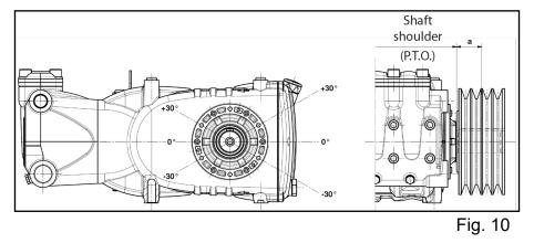
C) Pull the belts according to manufacturer instructions. Excessive pulling can cause reduced bearing life and wear out the pulley prematurely. Pulling depends on different variables as indicated in par. 9.12.
