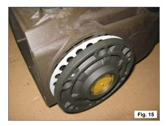
Once the type and number of shims have been determined using the table, check the following: assemble the shim pack on the indicator side cover centering (Fig. 15), secure the cover to the casing, following the procedure in par. 2.1.2, and tighten the screws to their recommended torque.
