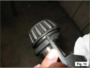
The new bearings can be mounted cold with a press or rocker, supporting it on the lateral surface of the ring nuts involved in press fitting with the rings. The fitting operation could be facilitated by heating the parts involved at a temperature between 250° - 300 °F (120° - 150 °C), making sure that the ring nuts are fully fitted in their respective seats.
