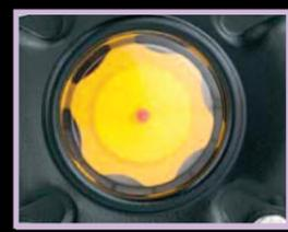
Large diameter of sight glass means easier oil checking
