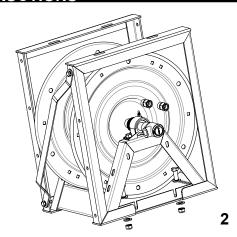
2) Bolt your hose reel to the ASSEMBLY FRAME/BRACE assembly. Use (4) M12 nuts and bolts and (8) M12 washers. Make sure the hose reel outlet (where the hose connects) faces away from the BRACE.
