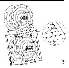
3) Bolt your second hose reel the ASSEMBLY FRAME/BRACE/ HOSE REEL assembly. Again, use (4) M12 nuts and bolts and (8) M12 washers.
