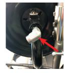
4. Attach 90° elbow (3/8"NPT-F x 3/8"NPT-F) to inlet fitting. Be sure elbow is clocked as shown (approximately 315° from post)
