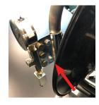
2. Secure manifold bracket with (2) M8 nuts and bolts.
